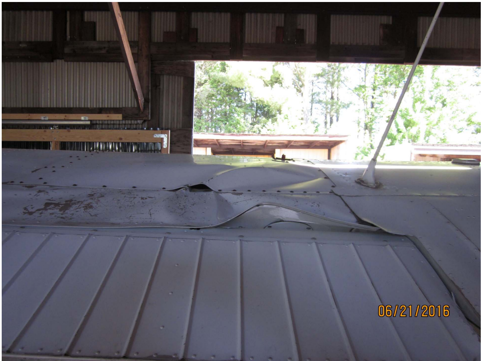
Photo 1 – View of Wing Damage after Recovery (FAA)
