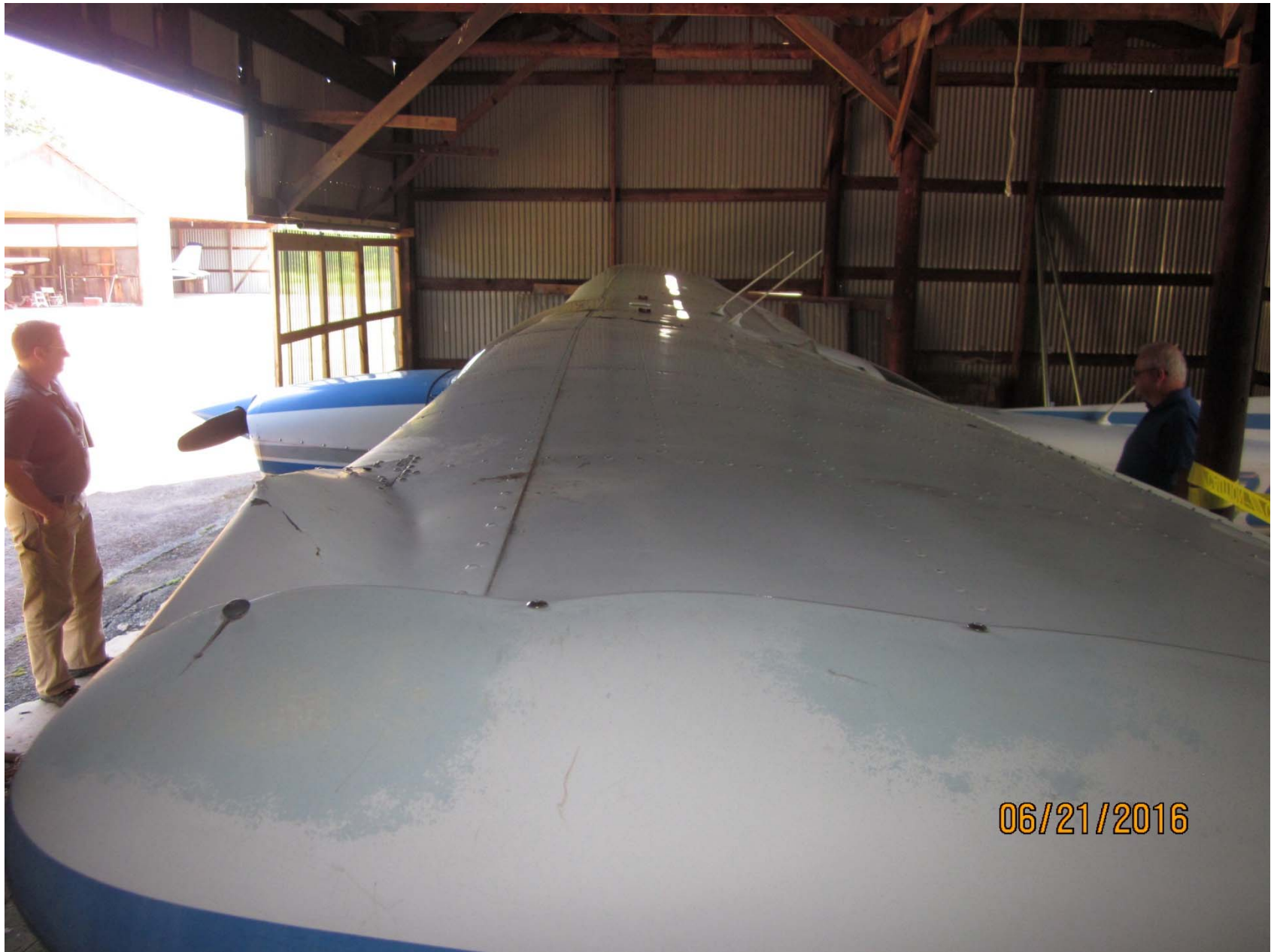
Photo 2 – View of Left Wing Damage after Recovery (FAA)
