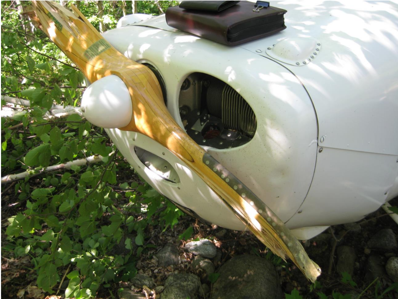
Photo 5 – View of propeller damage. Note both blades are splintered on the outboard sections. (Courtesy of FAA)
