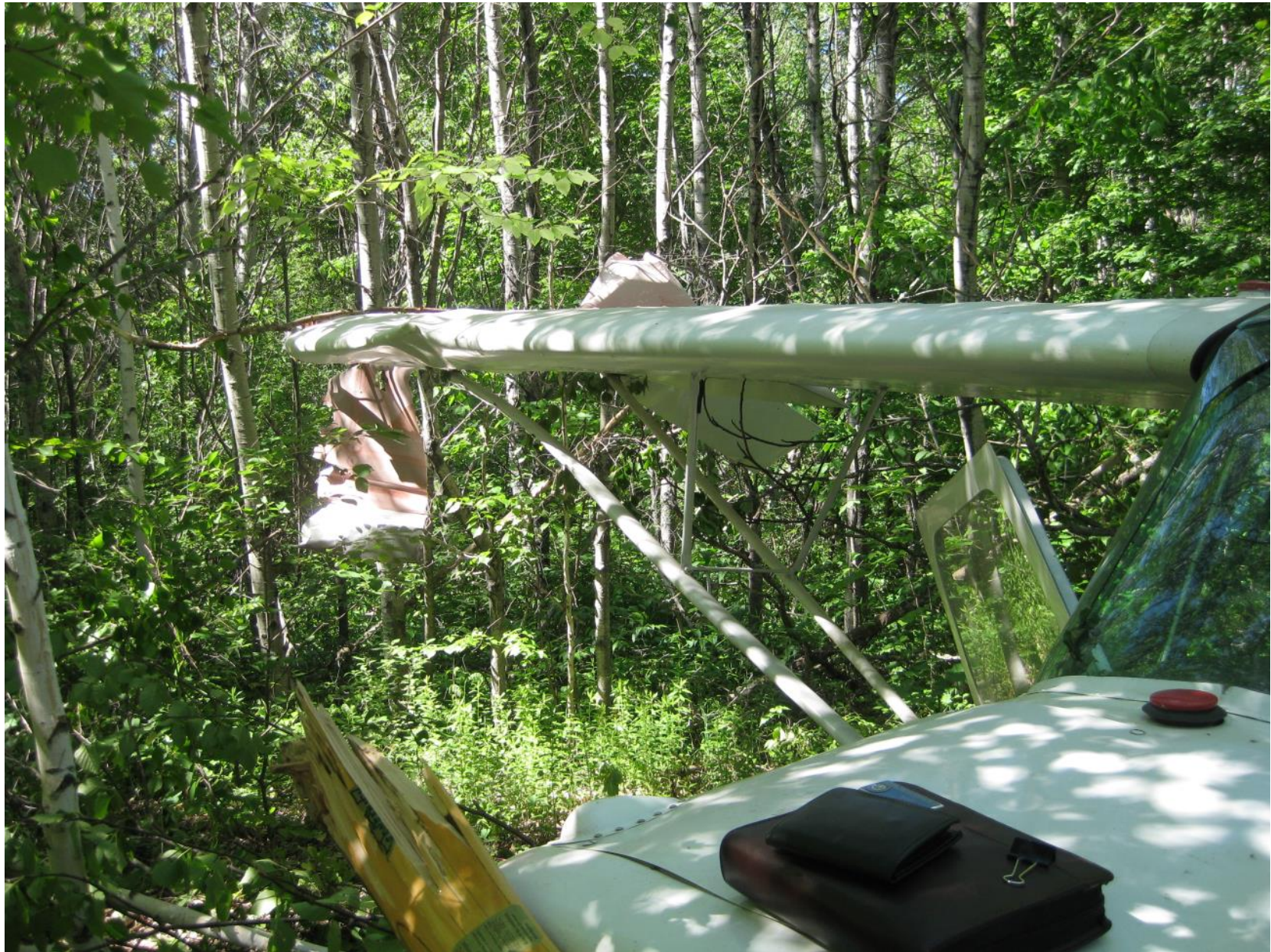
Photo 3 – View of right wing and strut damage. (Courtesy of FAA)
