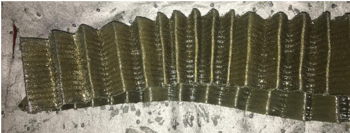
Picture 14. View of oil filter with metallic particles.
