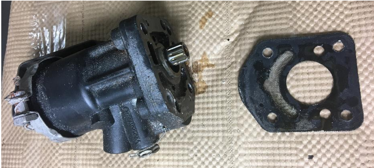
Picture 4. View of Propeller Governor with Oil Screen Removed.
