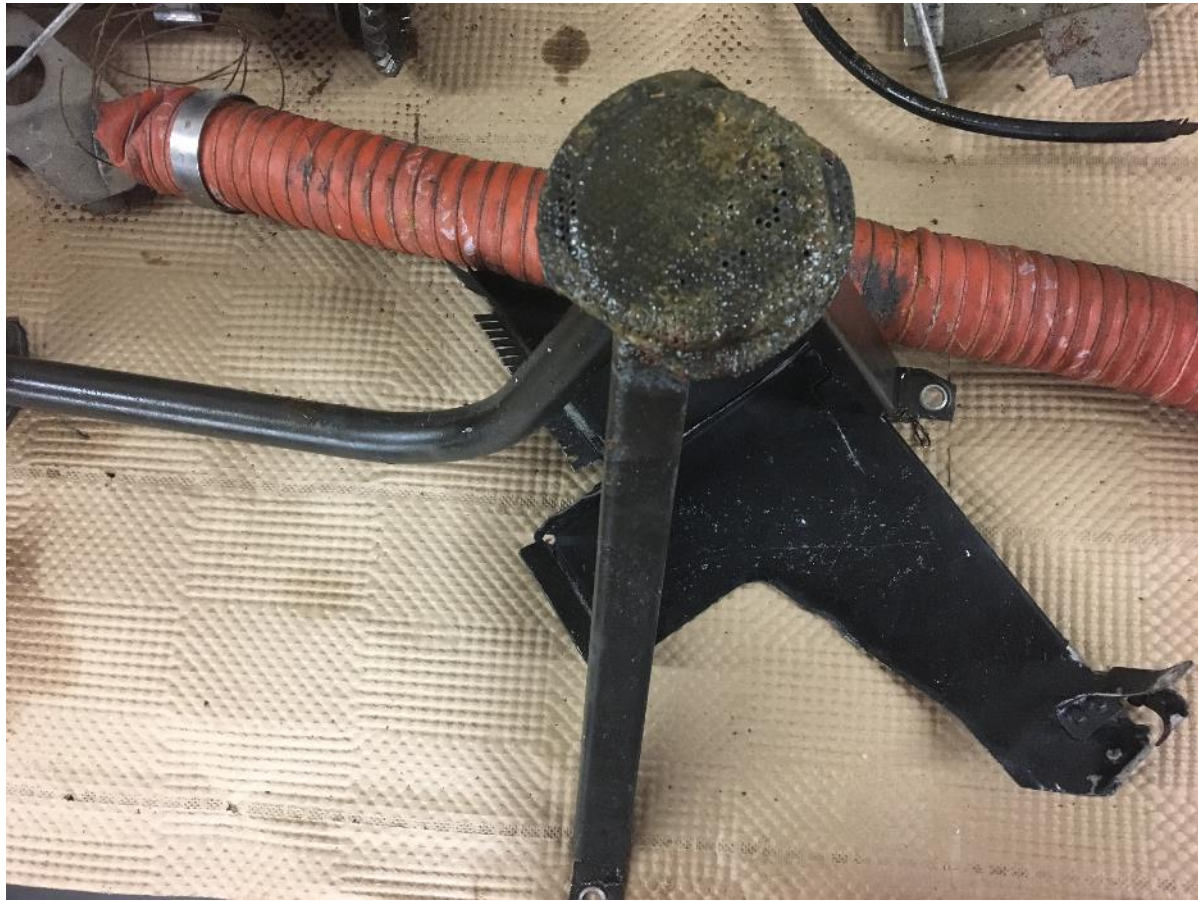
Picture 10. View of oil suction screen.
