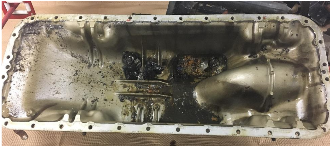
Picture 9. View of Oil Sump and Metallic Particles
