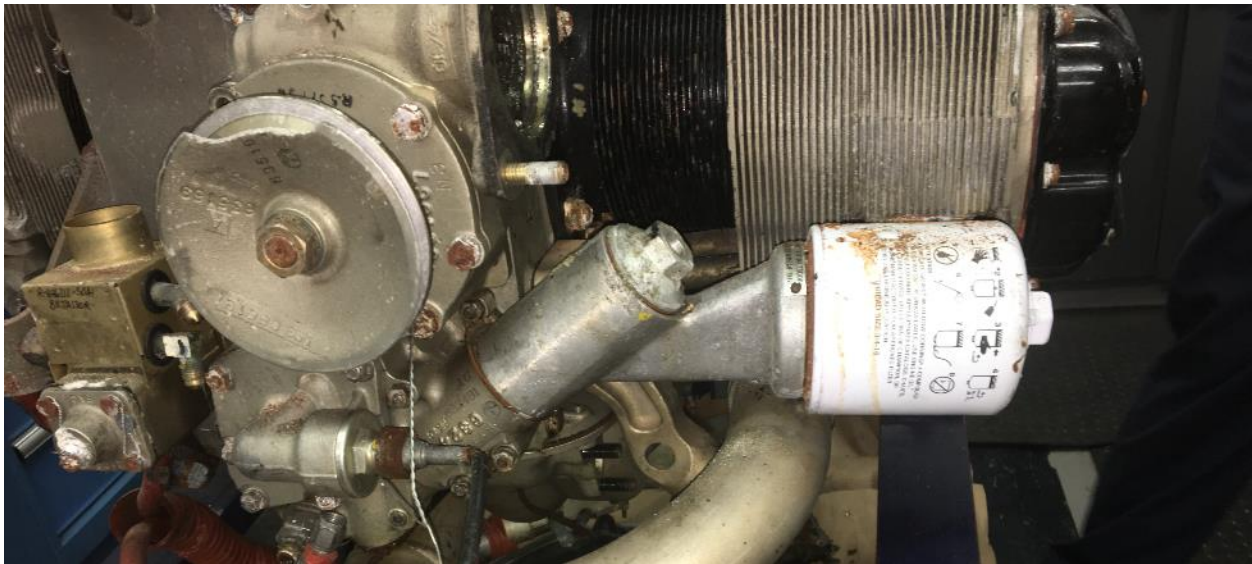
Picture 11. Oil filter installed on oil filter adaptor.
