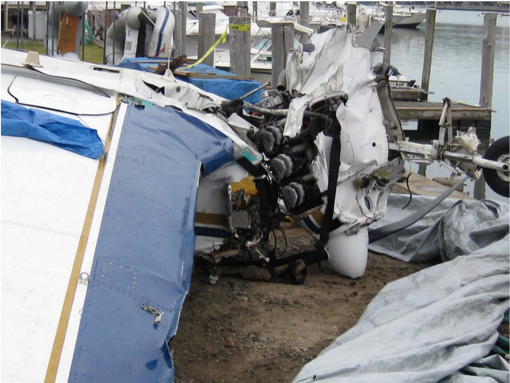
Photo 2 – View of engine after recovery (Courtesy of FAA)
