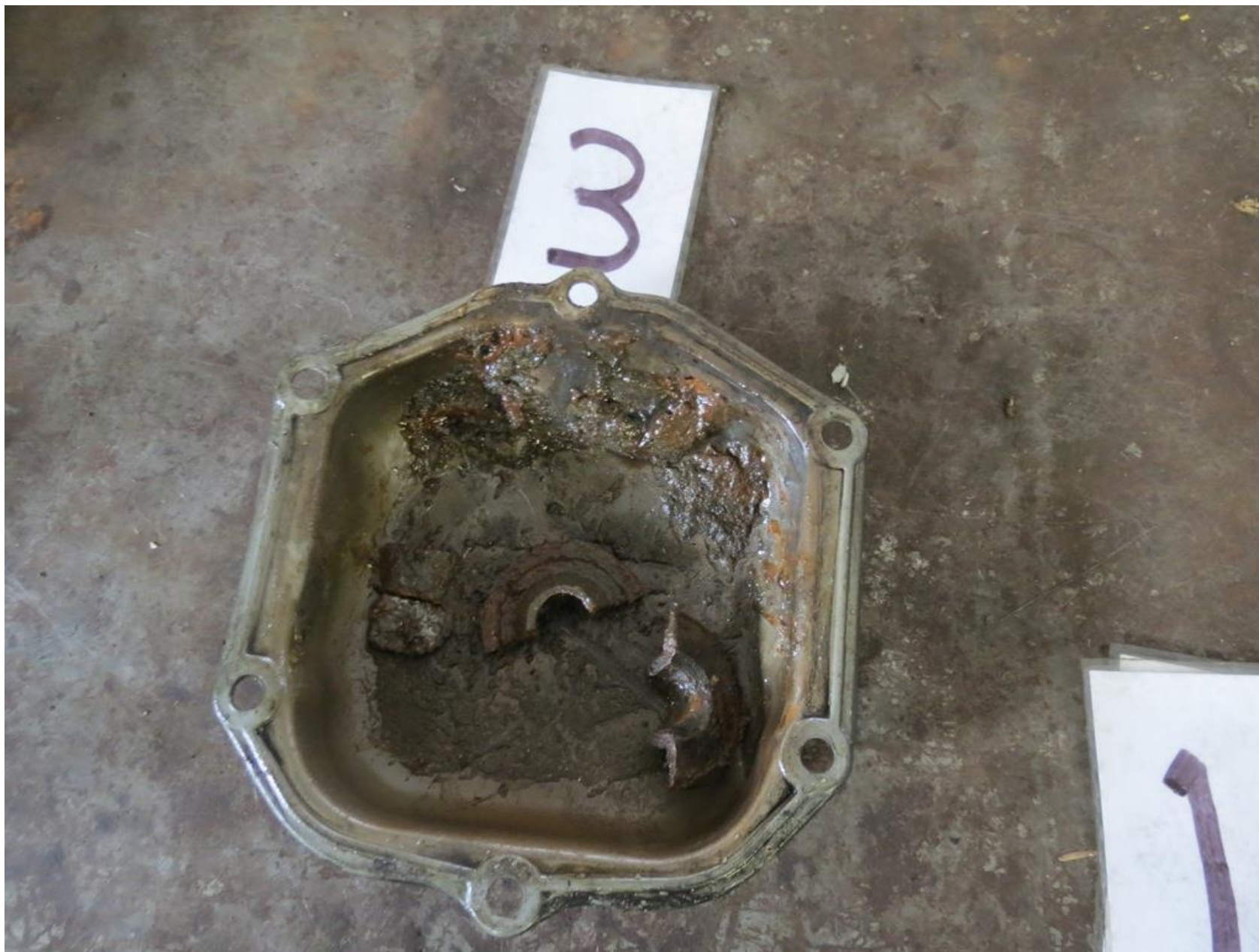
Photo 7 – Fractured No. 3 Valve Seat (Photo Courtesy of Lycoming)
