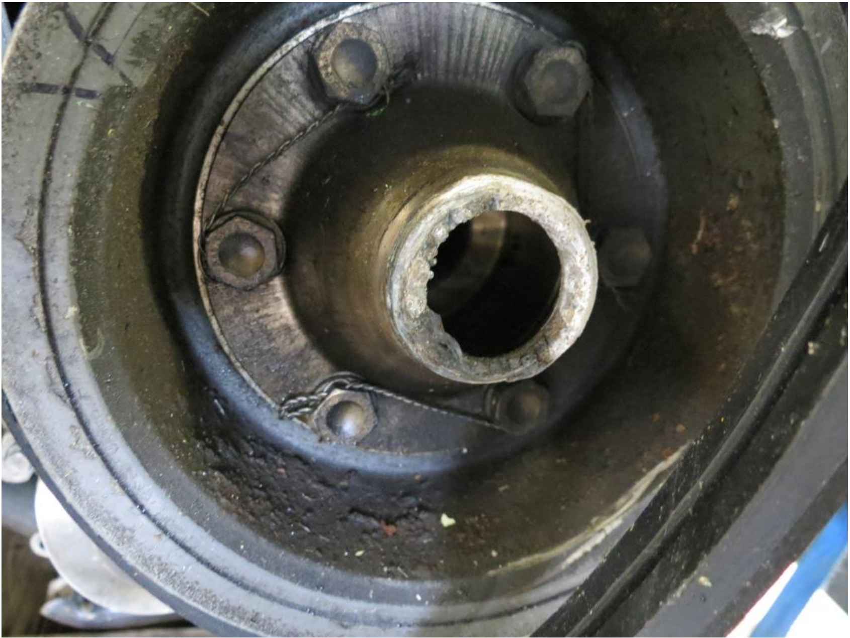
Photo 3 – Lower Drive Sheave With Dry And Caked on Grease (Photo Courtesy of Lycoming)
