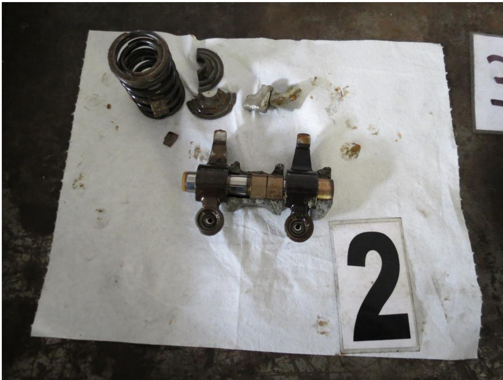
Photo 5 – Fractured No. 2 Valve And Bosses (Photo Courtesy of Lycoming)
