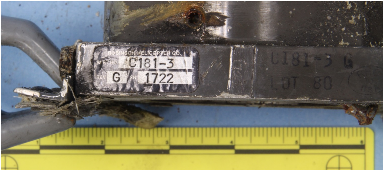
Figure 2 – The markings on the flange of the bearing assembly, as received.
