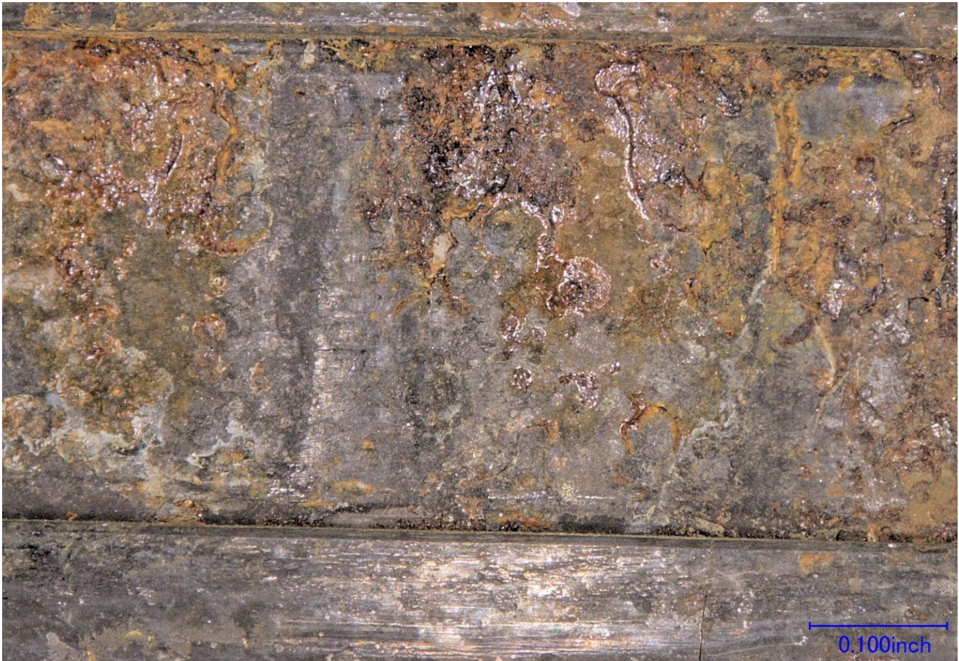
Figure 15 – Closer view of the inner race channel from Figure 14, showing sliding wear marks with a roller.
