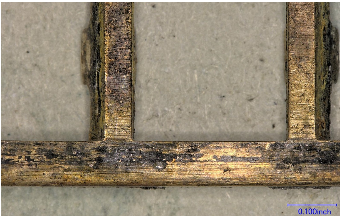
Figure 11 – The inner surface of the forward bearing cage, showing circumferential sliding wear, consistent with contact with the inner race.
