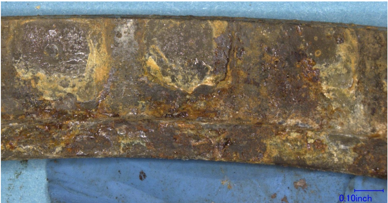
Figure 6 – Inner surface of the aft bearing outer race, as received. The depressions were consistent with the positions of the rollers while oxidation occurred.
