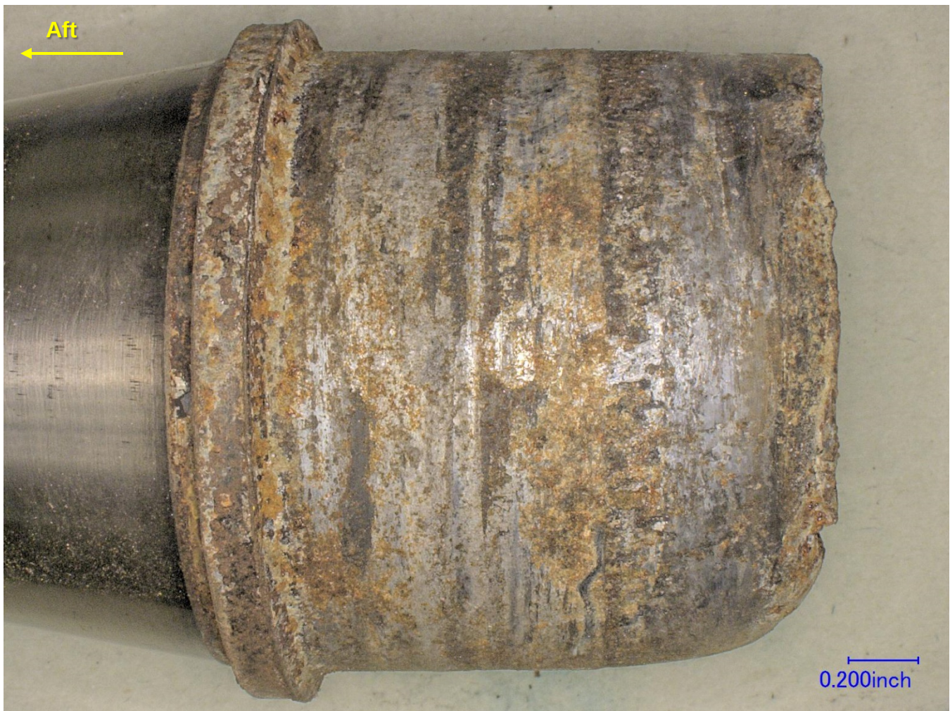
Figure 26 – Closer view of the aft side of the shaft, showing circumferential wear marks and deformation at the fracture.
