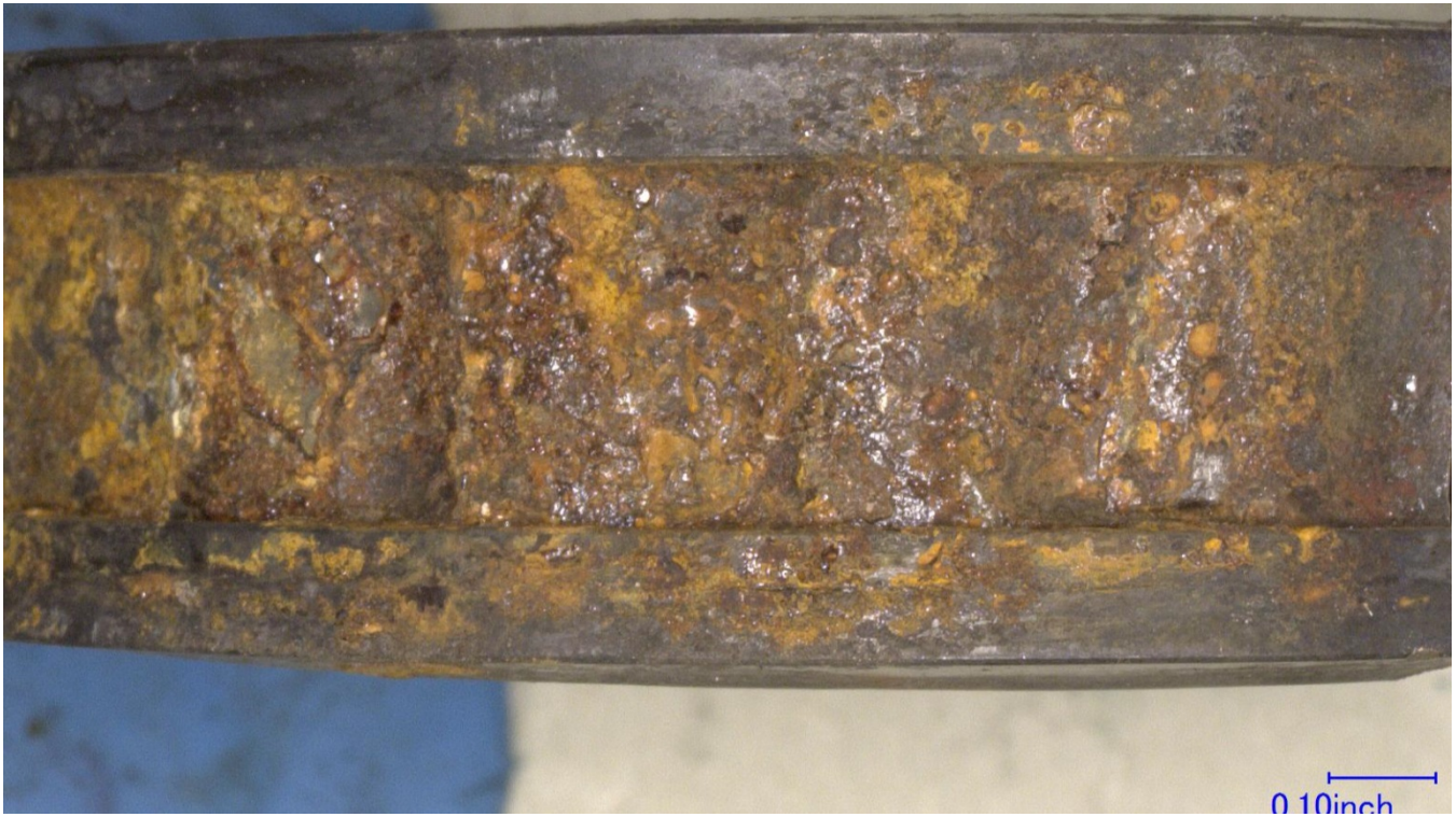
Figure 13 – The outer face of the inner race of forward bearing, showing dents and depressions consistent with the rollers, and deformation of the aft surface flange.
