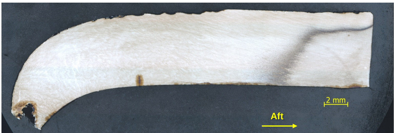
Figure 27 – BF optical metallograph cross section of the fracture surface of the aft shaft section (reversed from Figure 26). The fracture was located on the left (~500X, etched 2% Nital).
