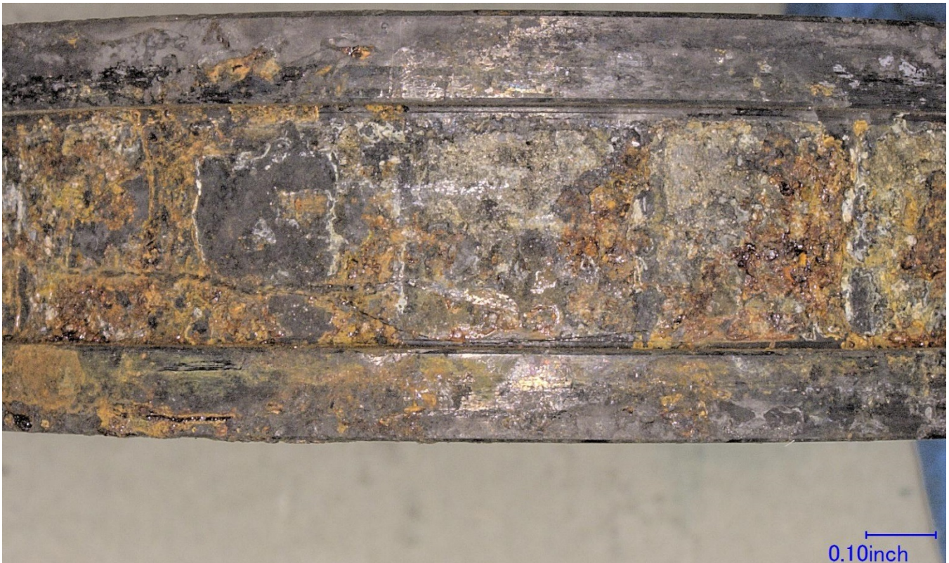
Figure 14 – The inner race of the forward bearing, after cleaning, showing deformation of the aft flange and roller depressions.
