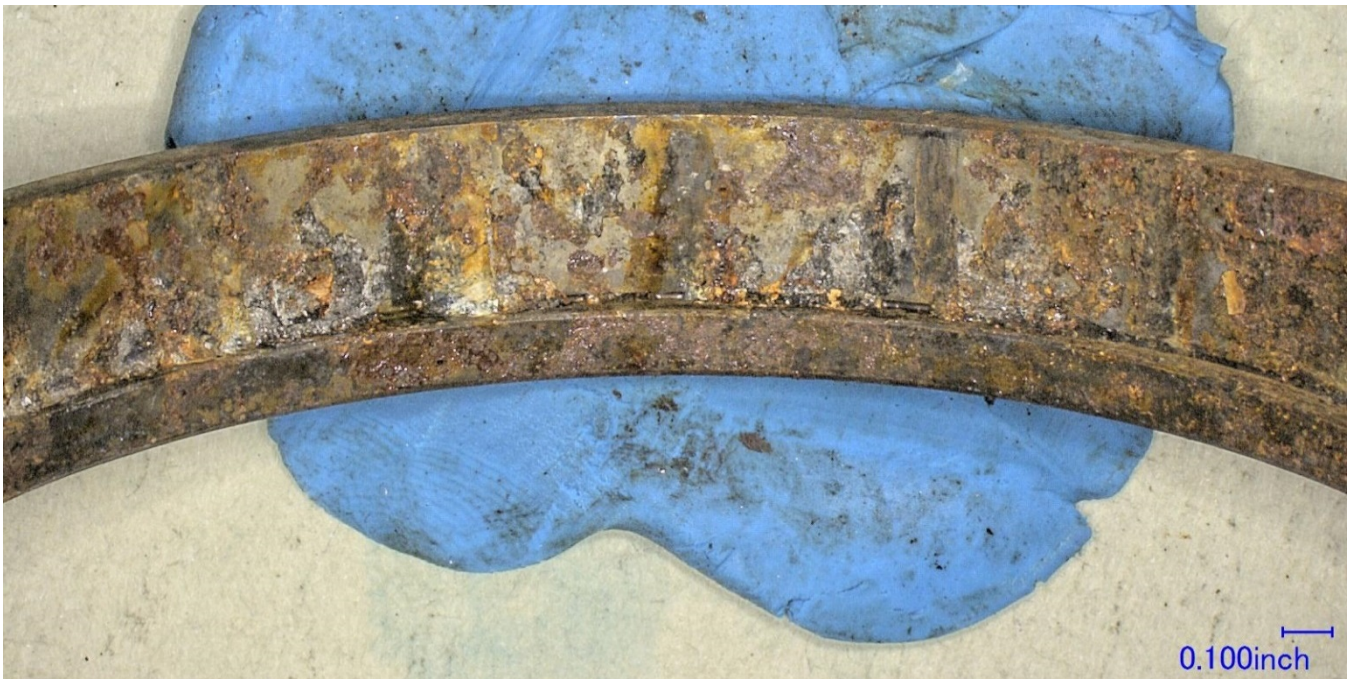
Figure 7 – The inner surface of the forward bearing outer race, after cleaning with acetone. The linear depressions were consistent with true brinelling of the race surface.
