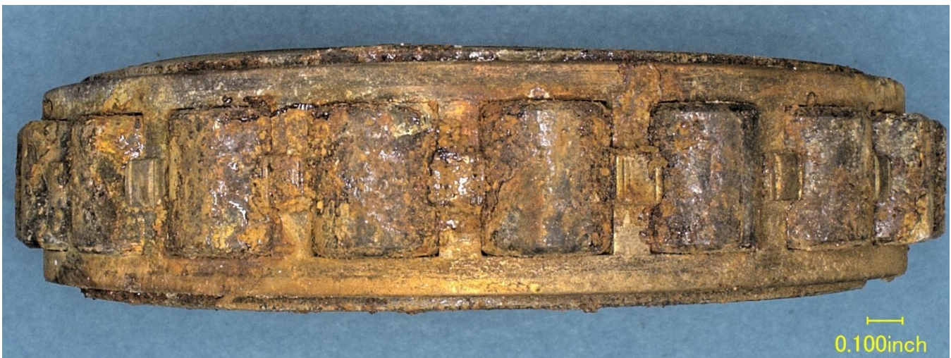
Figure 9 – A view of the forward bearing rollers, cage and inner race, viewed from outside, after cleaning with acetone.
