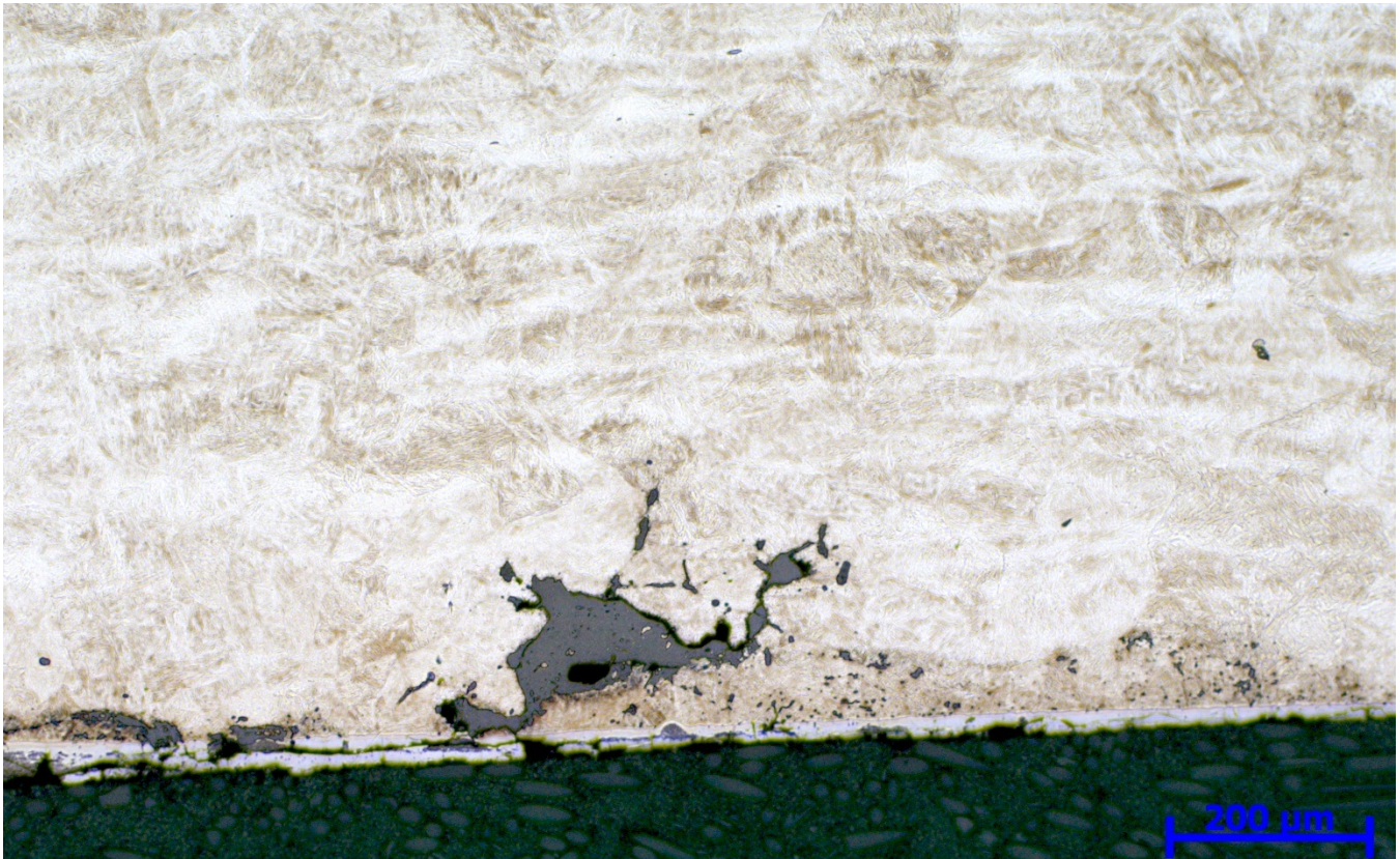
Figure 18 – BF optical metallograph of the forward bearing inner race inner surface, showing microstructure contrast and subsurface oxidation (~100X, etched 2% Nital).
