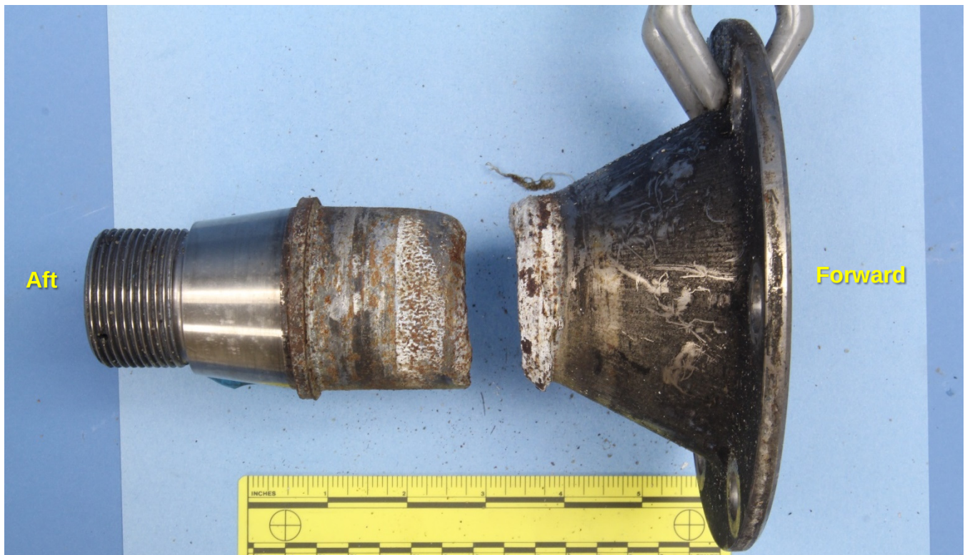
Figure 24 – The R44 shaft, showing the fracture location along the shaft taper, where the bearing assembly was positioned.
