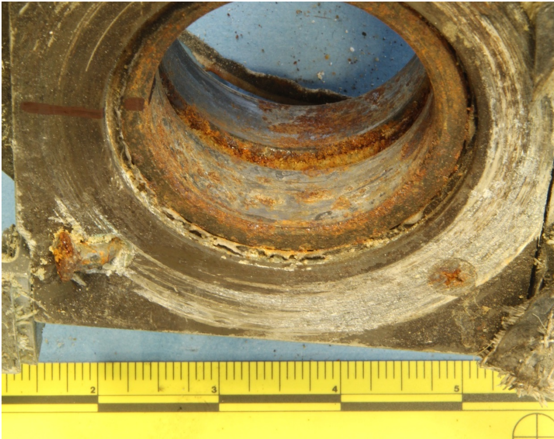
Figure 3 – The interior of the inner race of the aft side of the bearing. The 12 o'clock position was marked on the left side.
