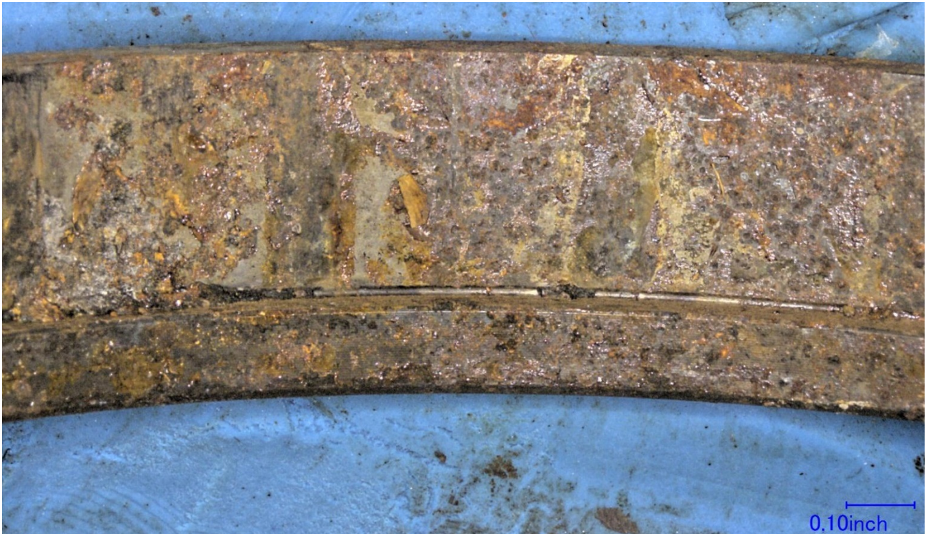
Figure 8 – A closer view of the brinelling depressions on the inner surface of the forward bearing race.
