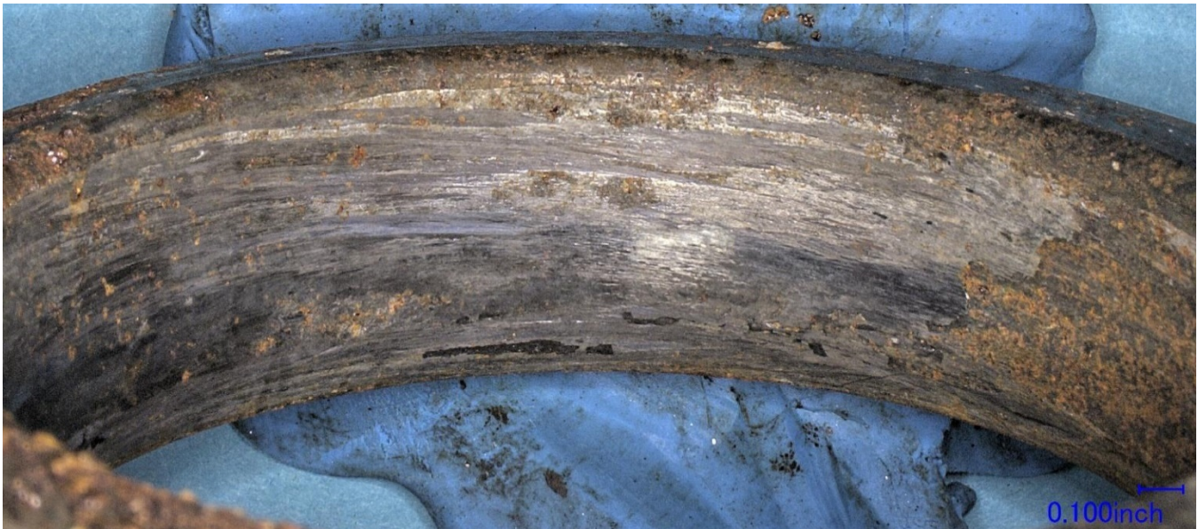
Figure 16 – The inner surface of the forward bearing inner race, showing circumferential wear and gouging.
