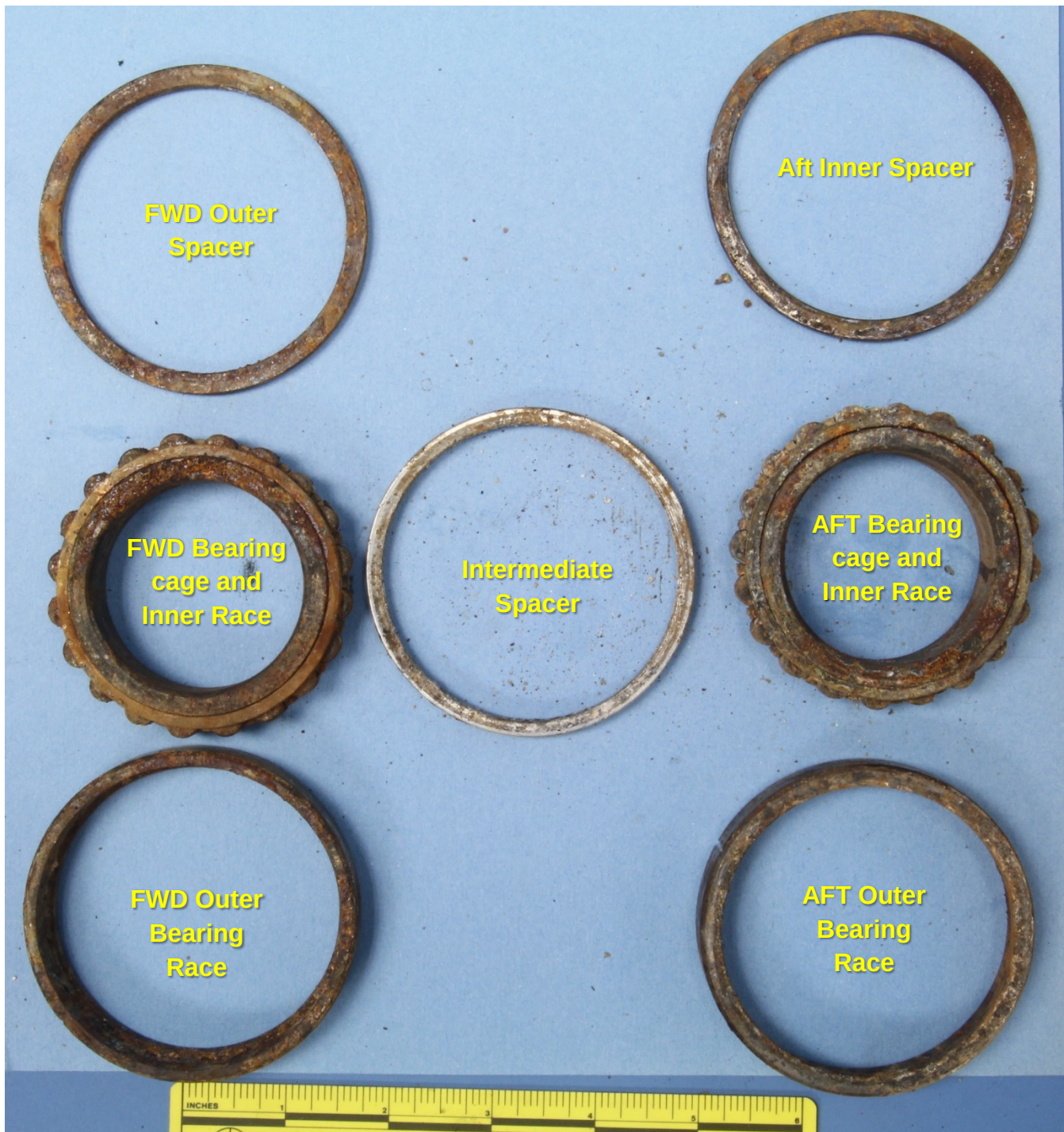
Figure 5 – The bearing components, after complete disassembly, ordered from forward side to aft side from left to right.
