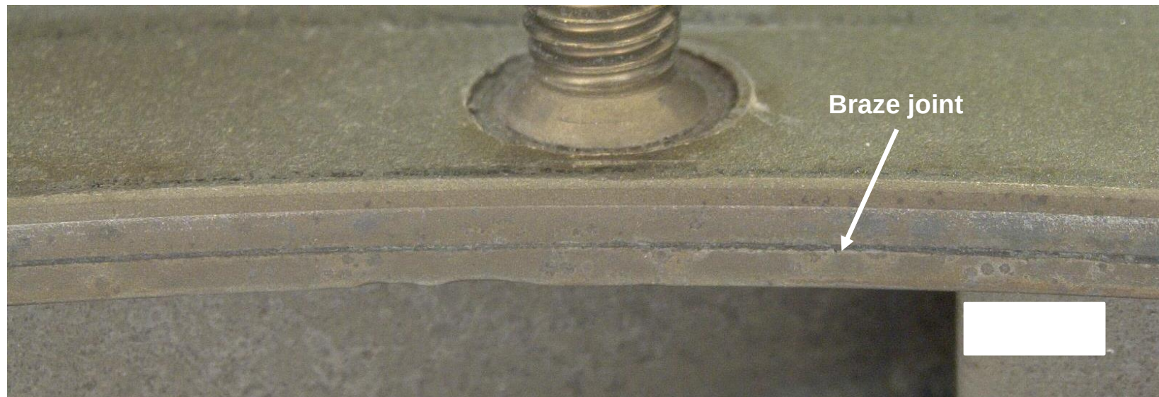
Figure 6. Radial views of the aft side of the compressor diffuser. The views are rotated approximately 90° from Figure 5. The bottom image (yellow boxed area) shows a detailed view of the inboard rim at the 180° position, which exhibited no evidence of voids or debonding at the inboard aft braze joint. The red boxed area is shown in more detail in Figure 8.
