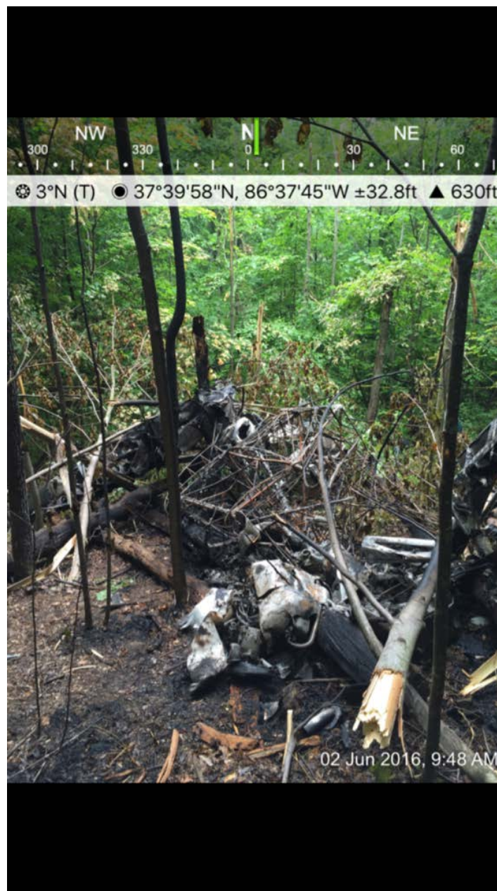
Photo 4 – FAA Digital Picture. View of the Main Wreckage at the Accident Site. Note the Fire Damage to the Wreckage and Surrounding Area.
