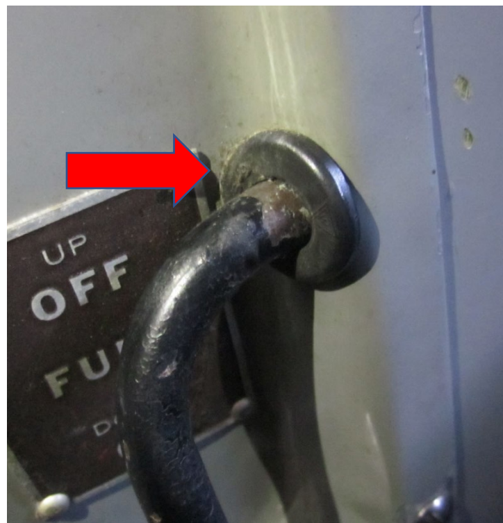
Exemplar Airplane Fuel Shutoff (Note: Installed Grommet)
