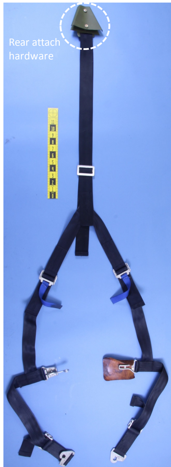
Figure 1 As-received rear-seat shoulder-harness and rear attach-hardware assembly.
