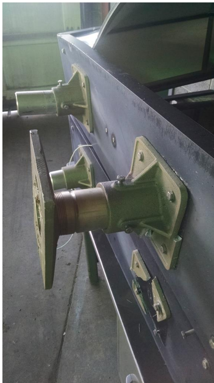
Photo 8 - FAA Digital Photograph. View Depicting 1 Non-Fractured Frangible Post
