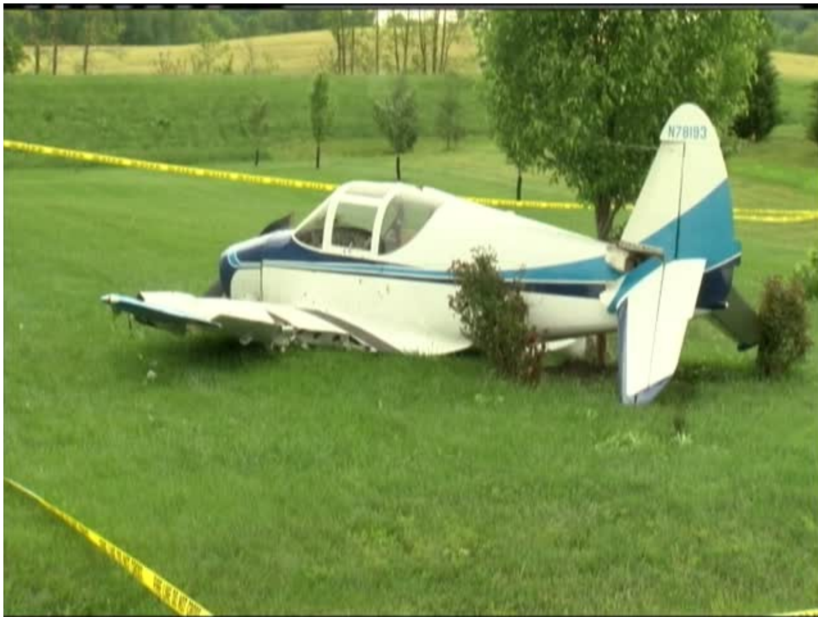
Photo 1 – Witness photo-View of airplane wreckage showing damage to wings, fuselage and empennage.
