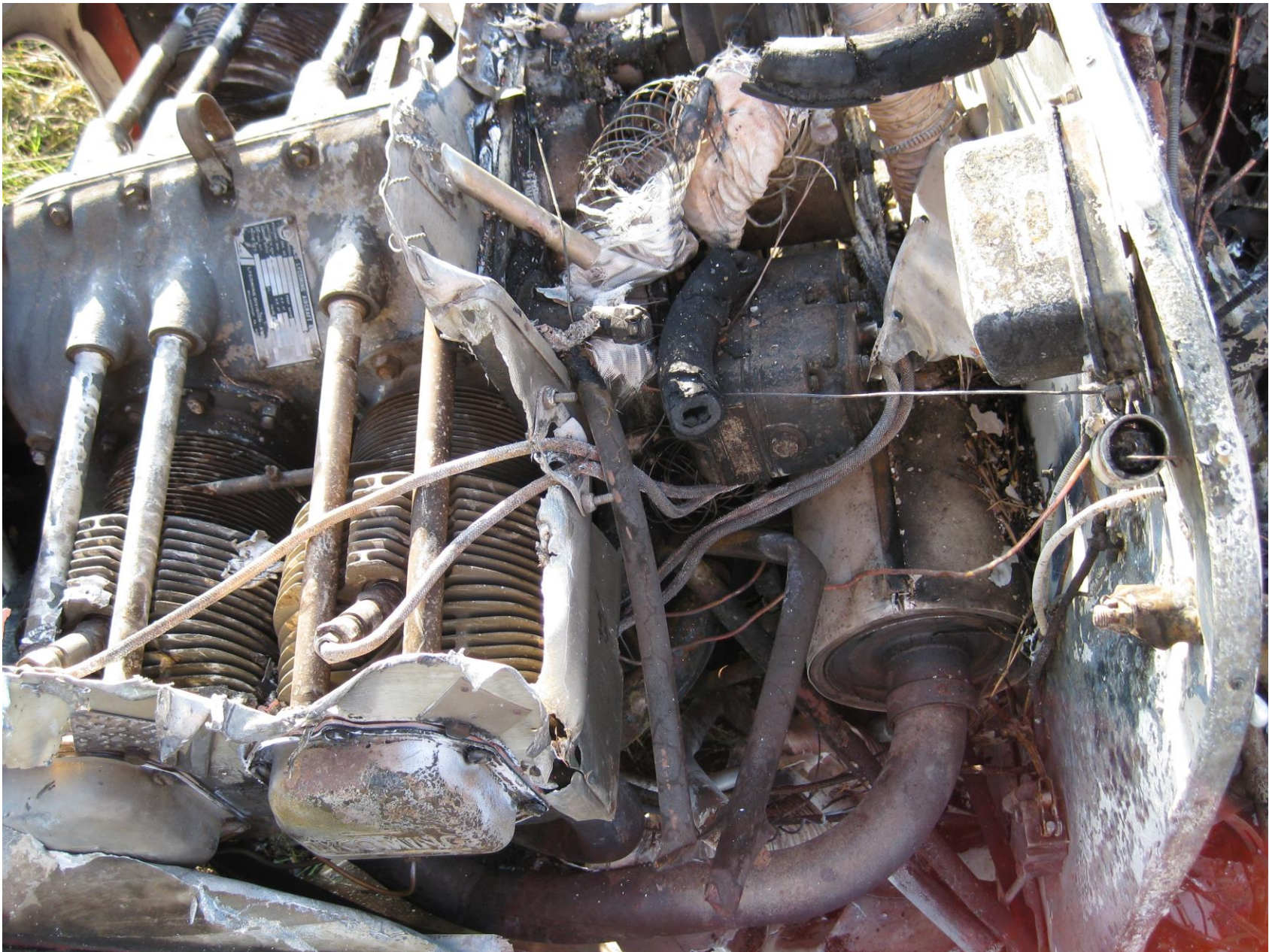
Photo 3 – Damaged Engine with Bird Nest Remnants Near Manifold and Firewall
