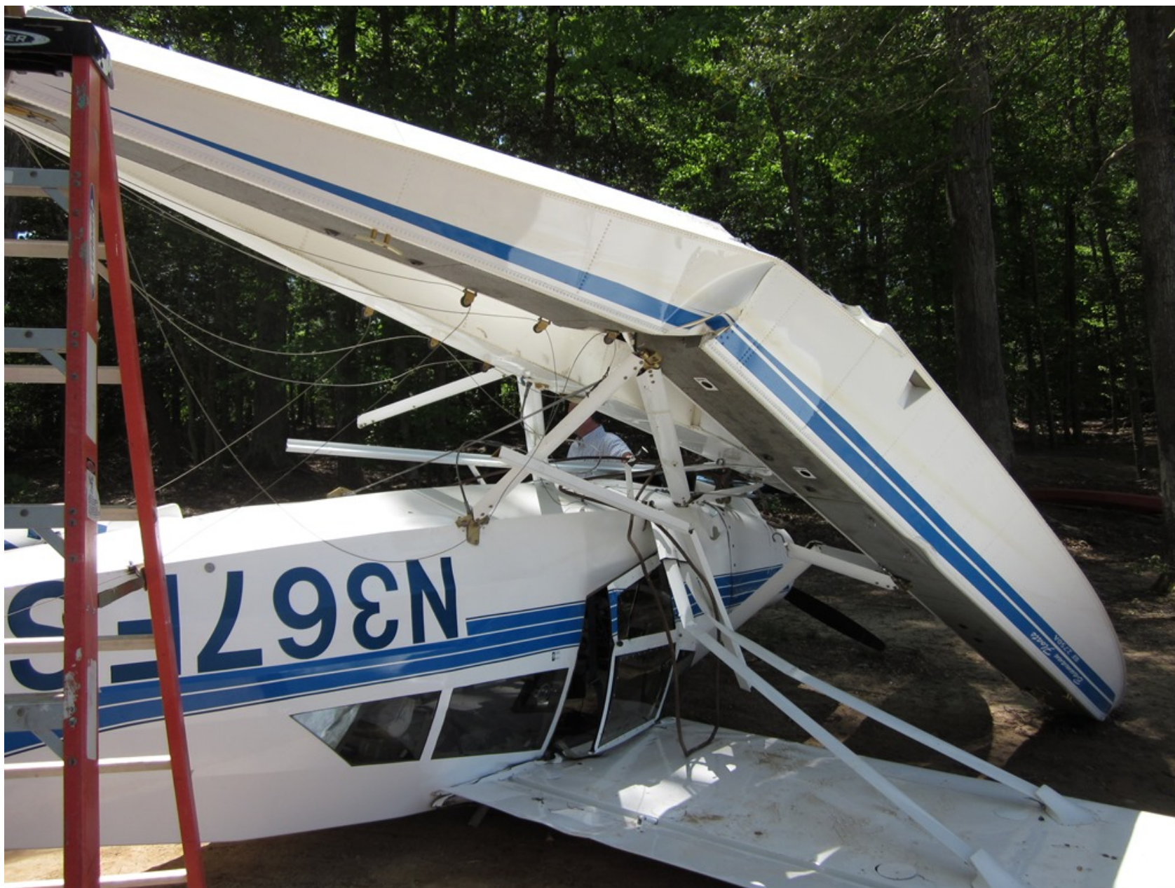
Photo 2 – View of Left Float Damage (Courtesy of FAA)
