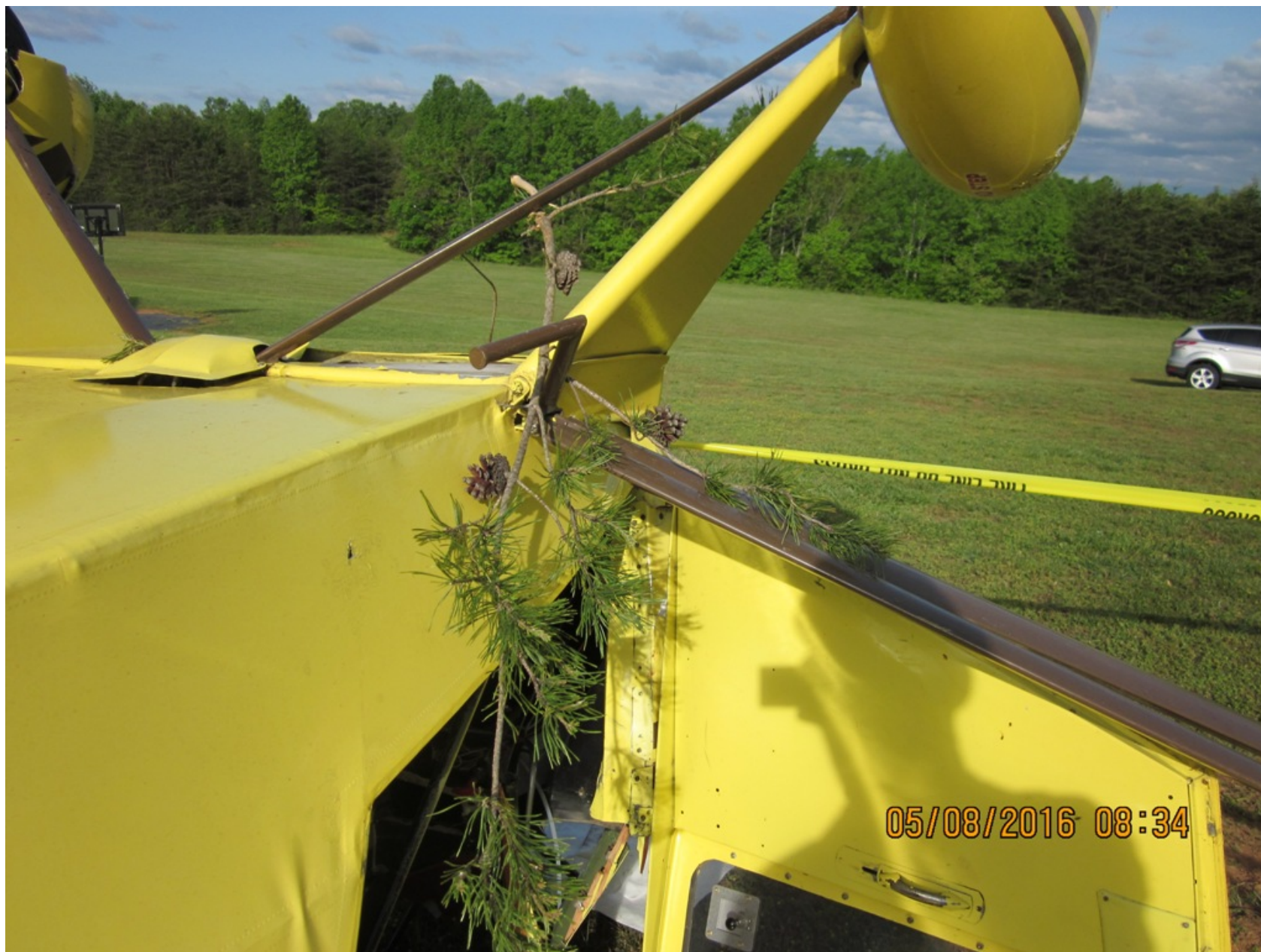
Photo 2 - FAA Digital Photograph. View Depicting the Inboard Portion of the Fuselage Adjacent to the Cockpit. Note the Tree Limb near the Wing Strut
