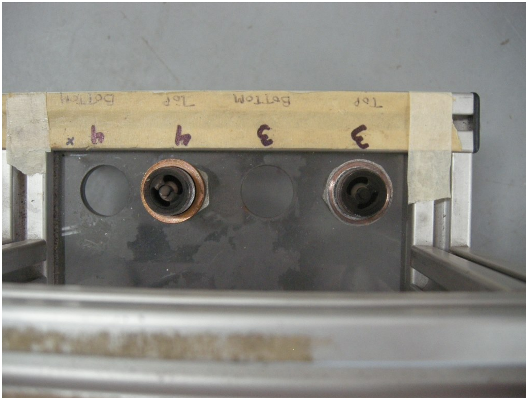
Photo 5 – Numbers 3 and 4 Spark Plugs (NTSB Photo)
