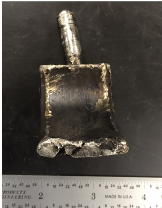
Figure 3 Fractured cap and bolt
