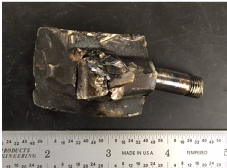
Figure 1 Fractured cap and bolt
