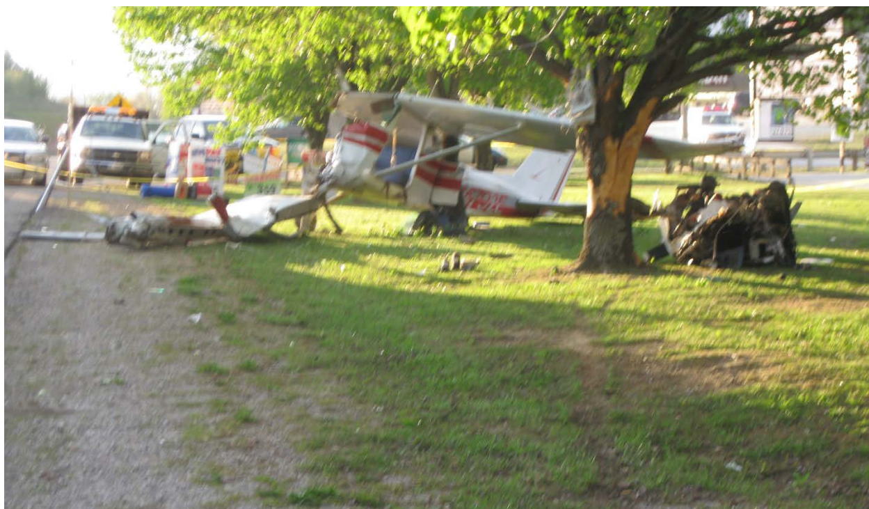
Figure 2 Left front view of the airplane and the separated engine to the right of the tree (Photo courtesy of the FAA)
