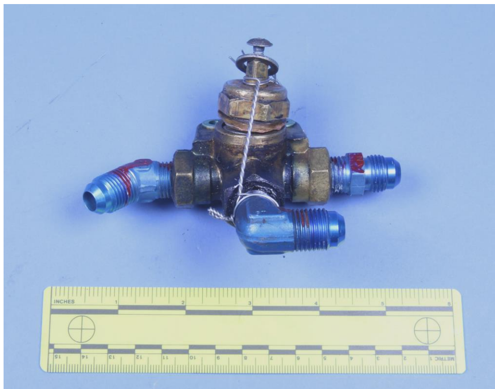
Figure 2: Fuel selector valve cap safety wired to valve body.
