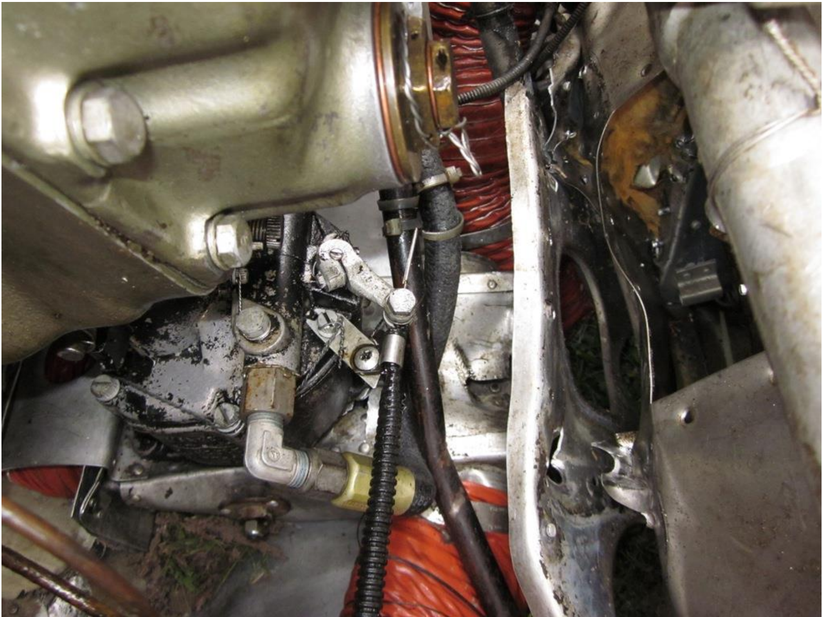
Photo 3 - FAA Digital Photograph. View Depicting the As-Found Position of the Mixture Control at the Carburetor in the Idle-Cutoff Position
