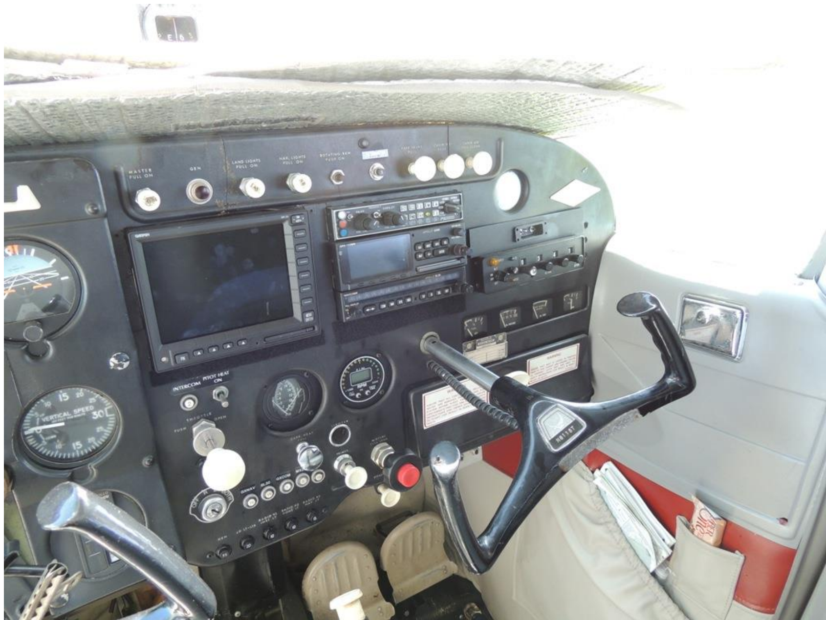
Photo 2 - FAA Digital Photograph. View Depicting the As-Found Position of the Mixture Control
