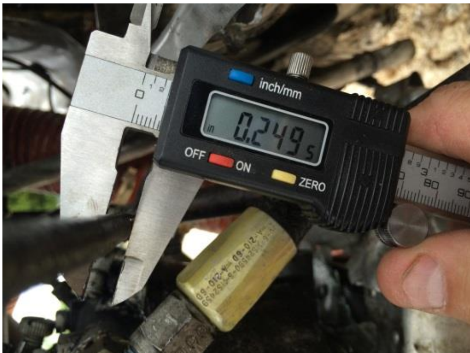
Figure 4: Measurement of plastic sheathing
