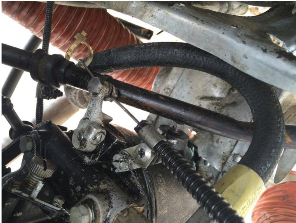
Figure 2: Mixture control sheathing installed in clamp for 1 st engine run
