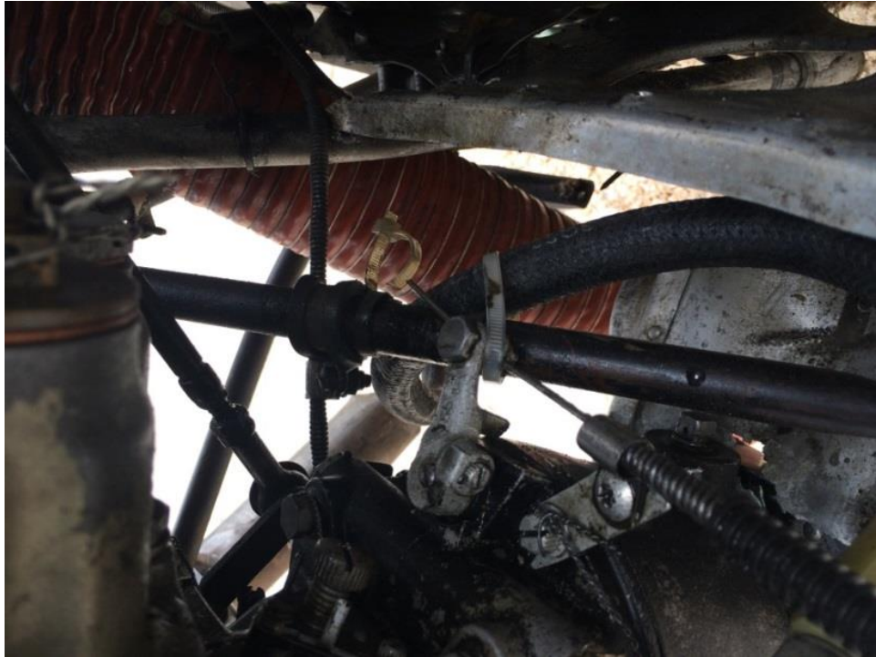
Figure 3: Mixture control fixed in full-rich for 3rd engine run
