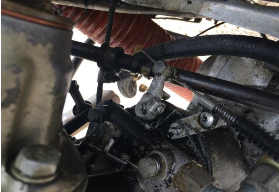
Figure 1: View of mixture cable, clamp, and sheathing as first viewed
