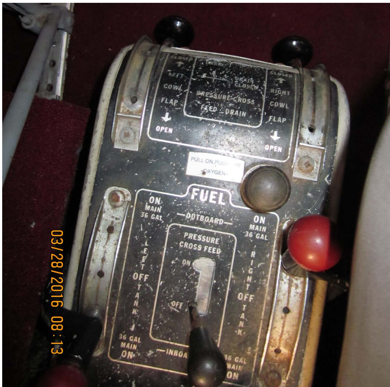
Figure 3 Fuel selector positions (Photo courtesy of FAA)
