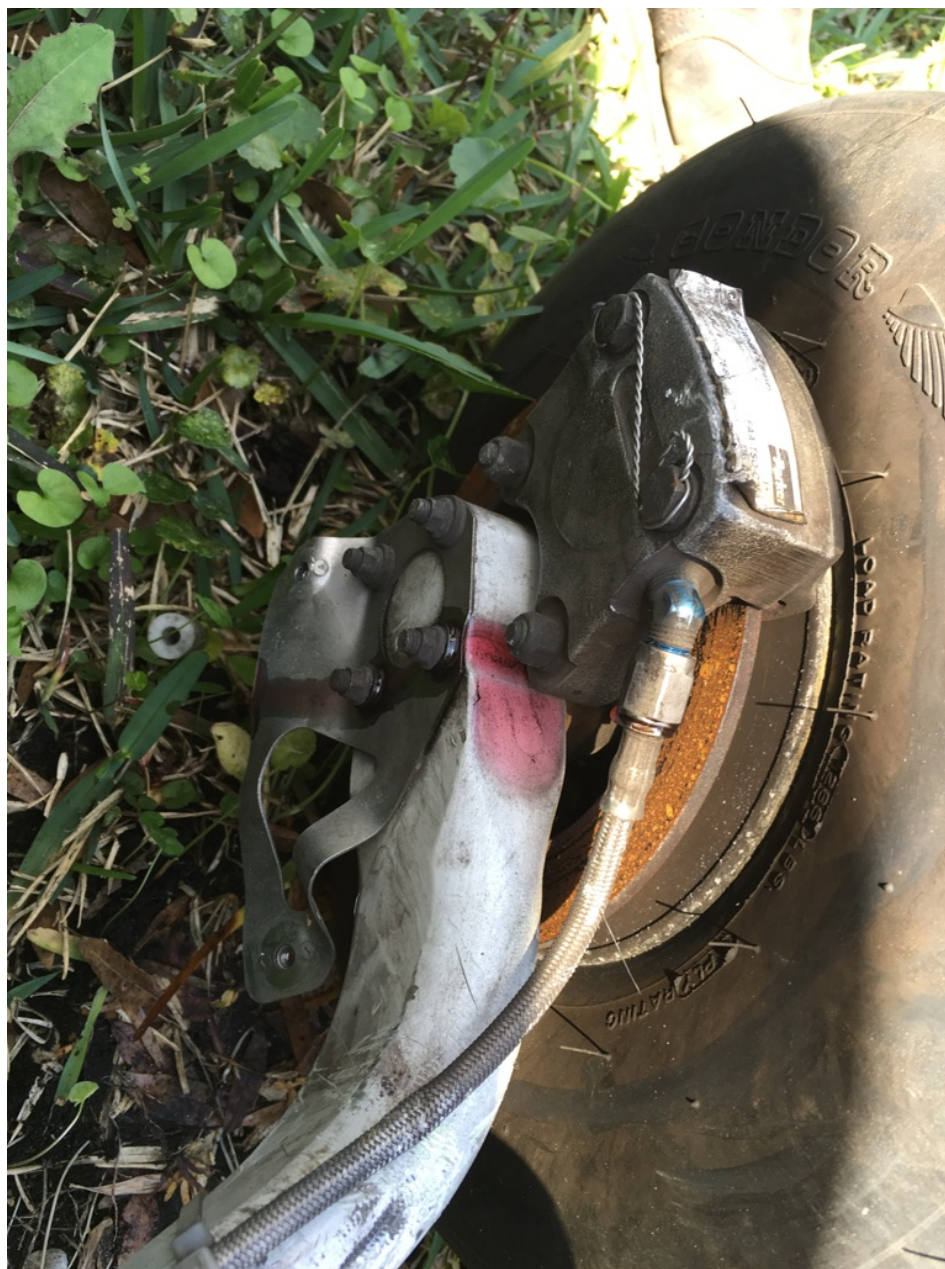
Photo 5 - FAA Digital Photograph. View Depicting Fluid Draining from Loosened Line at Left Brake Caliper
