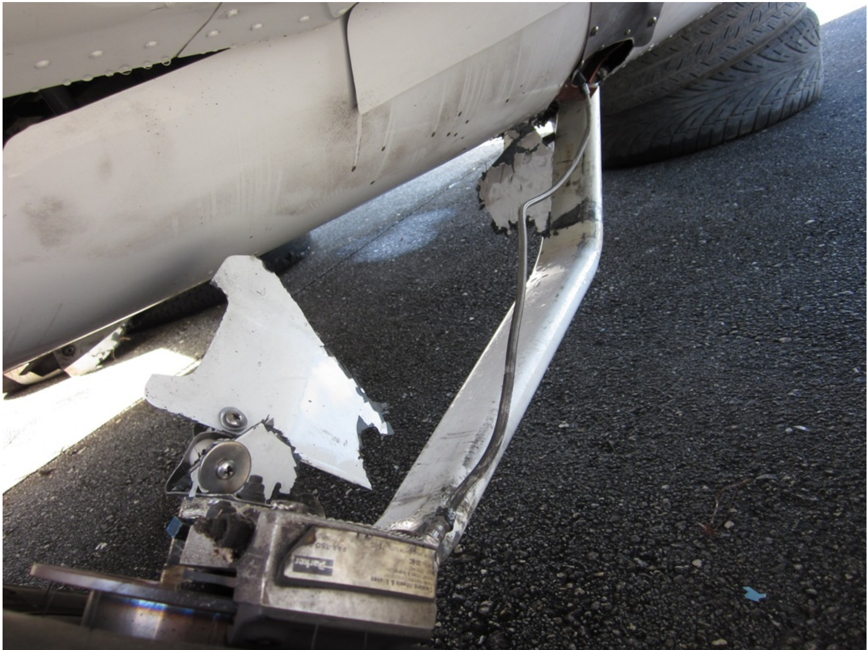
Photo 3 – FAA Digital Photograph. View Depicting the Right Main Landing Gear, Right Brake, and Right Brake Line Before Being Disconnected by Recovery Crew
