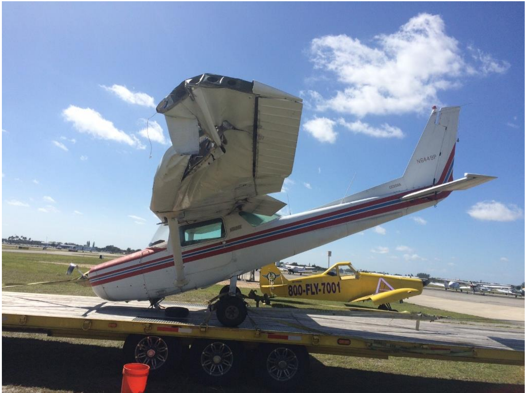
Photo 1 – FAA Digital Photograph. View Following Recovery Depicting the Damage to the Left Wing and Separated Nose Landing Gear
