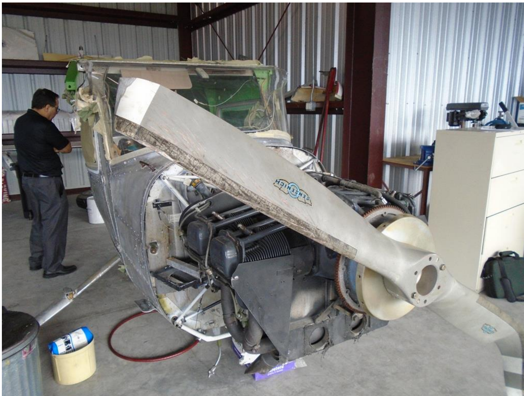
Photo 3 - FAA Digital Photograph. View Following Recovery Depicting the Damage To Other Propeller Blade
