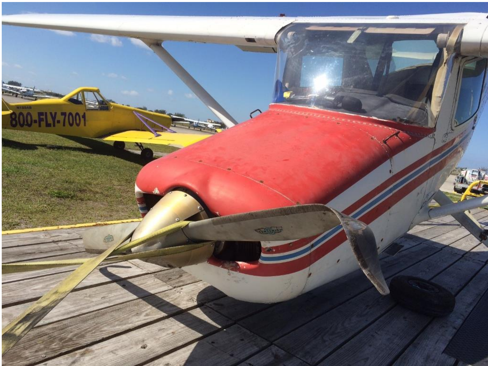
Photo 2 - FAA Digital Photograph. View Following Recovery Depicting the Damage To One Propeller Blade.
