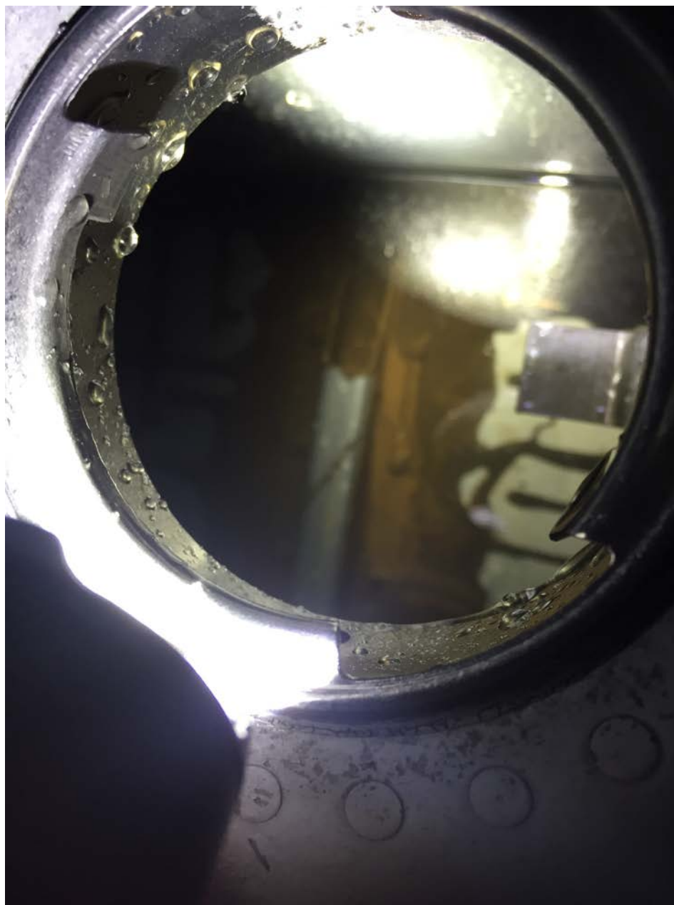
Photo 7 – Contents of Right Fuel Tank – Courtesy of FAA
