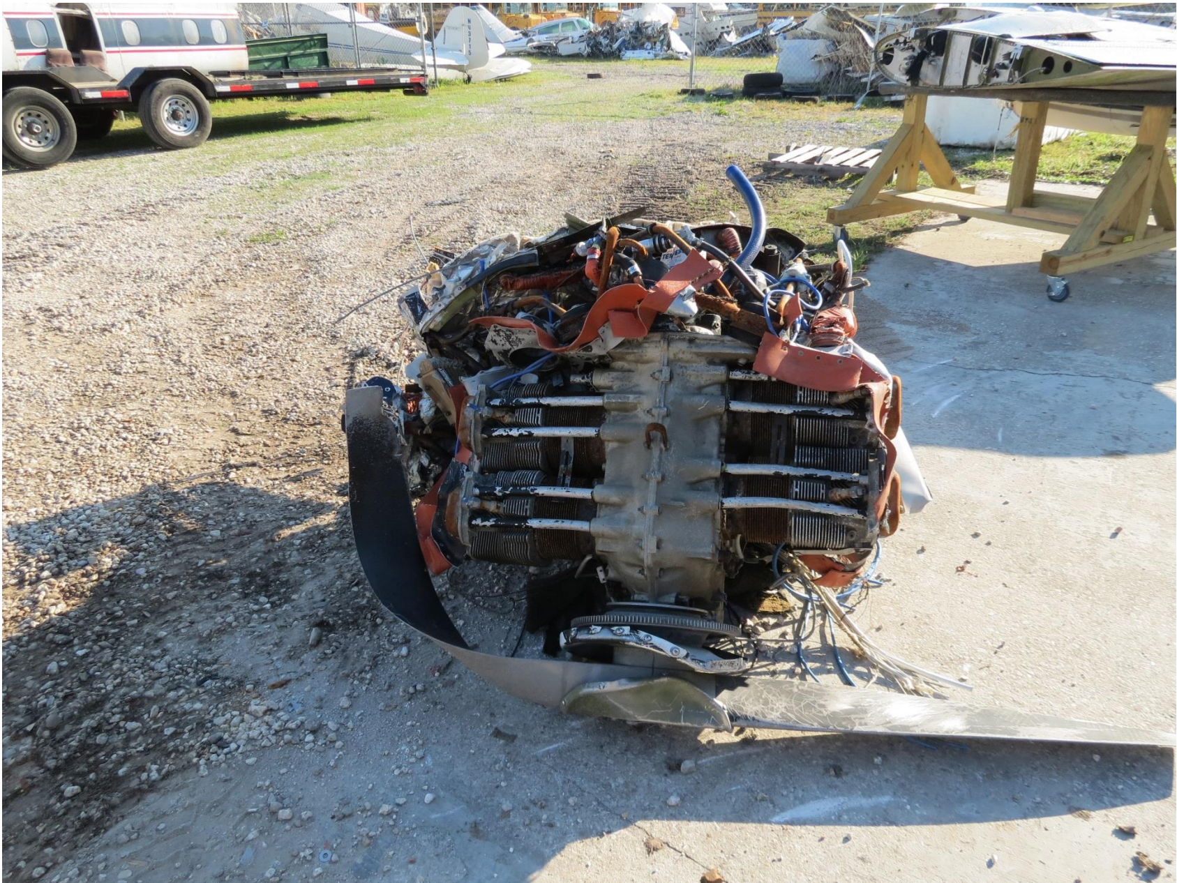
Photo 4 – View of Engine after Recovery (Lycoming)
