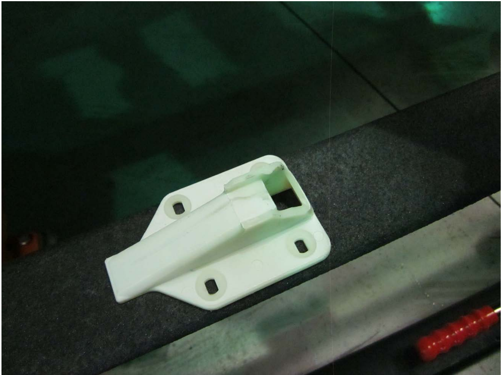
Photo 4 – View of broken door stop bracket
