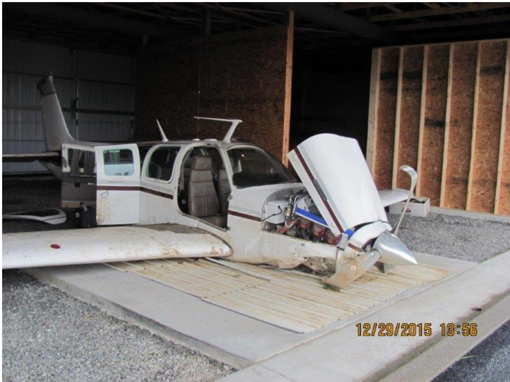
Photo 2 - View of front of airplane from right side showing nose damage
