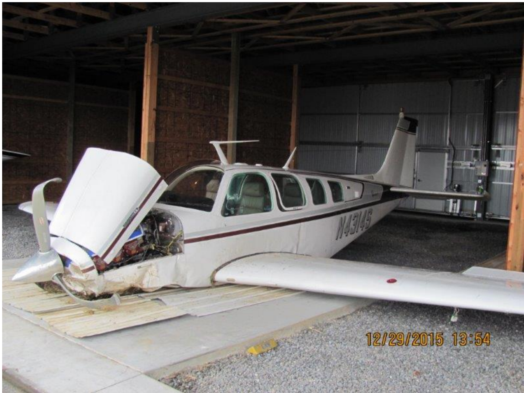
Photo 1 – View of front of airplane from left side showing nose damage
