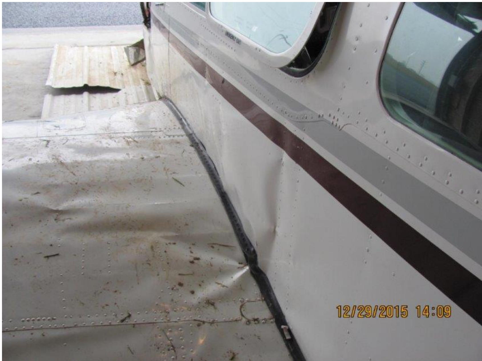
Photo 3 – View of left side of fuselage showing buckling at wing root
