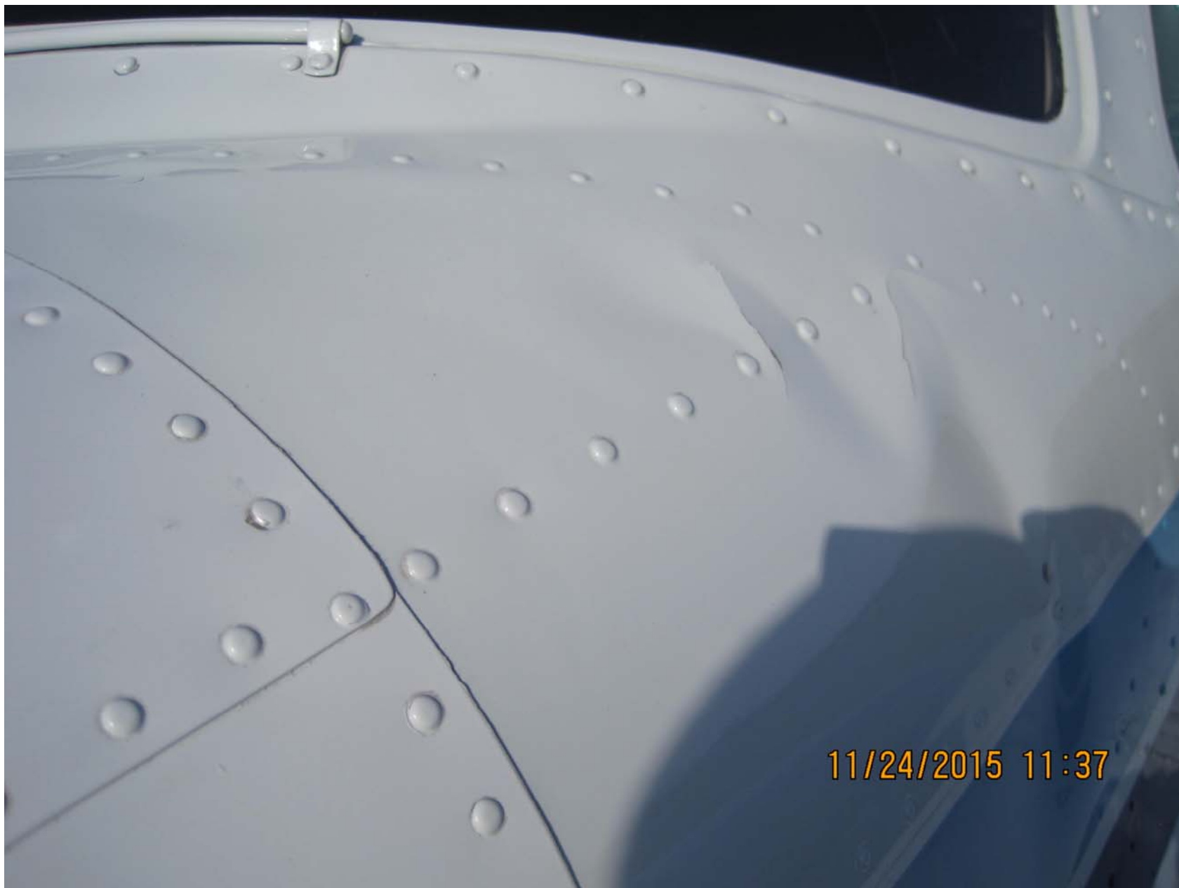
Photo 2 – View of Fuselage Damage (FAA)
