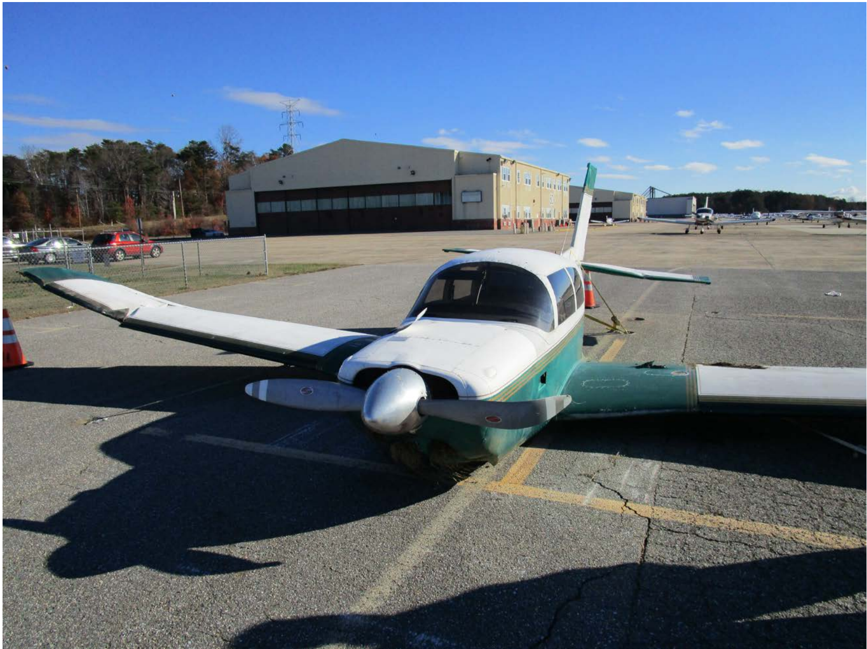
Photo 1 – Front view of airplane-revealing damage to left and right wings
