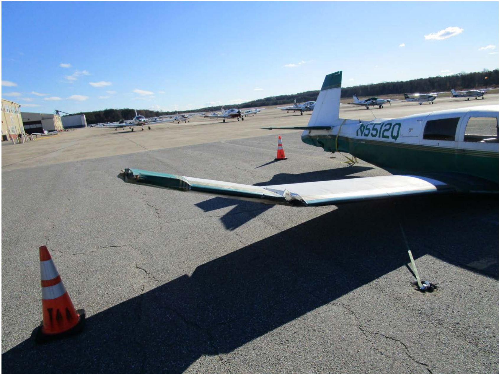
Photo 2 – View of right wing showing buckling upward
