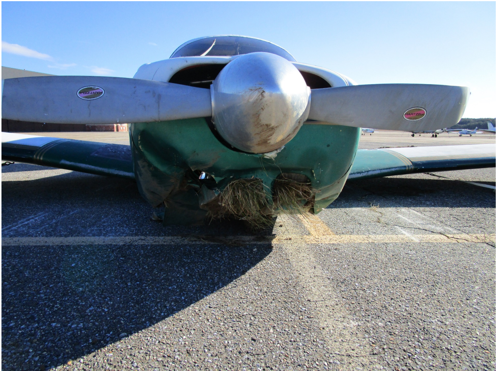
Photo 4- Front view underside of airplane showing damage to the firewall
