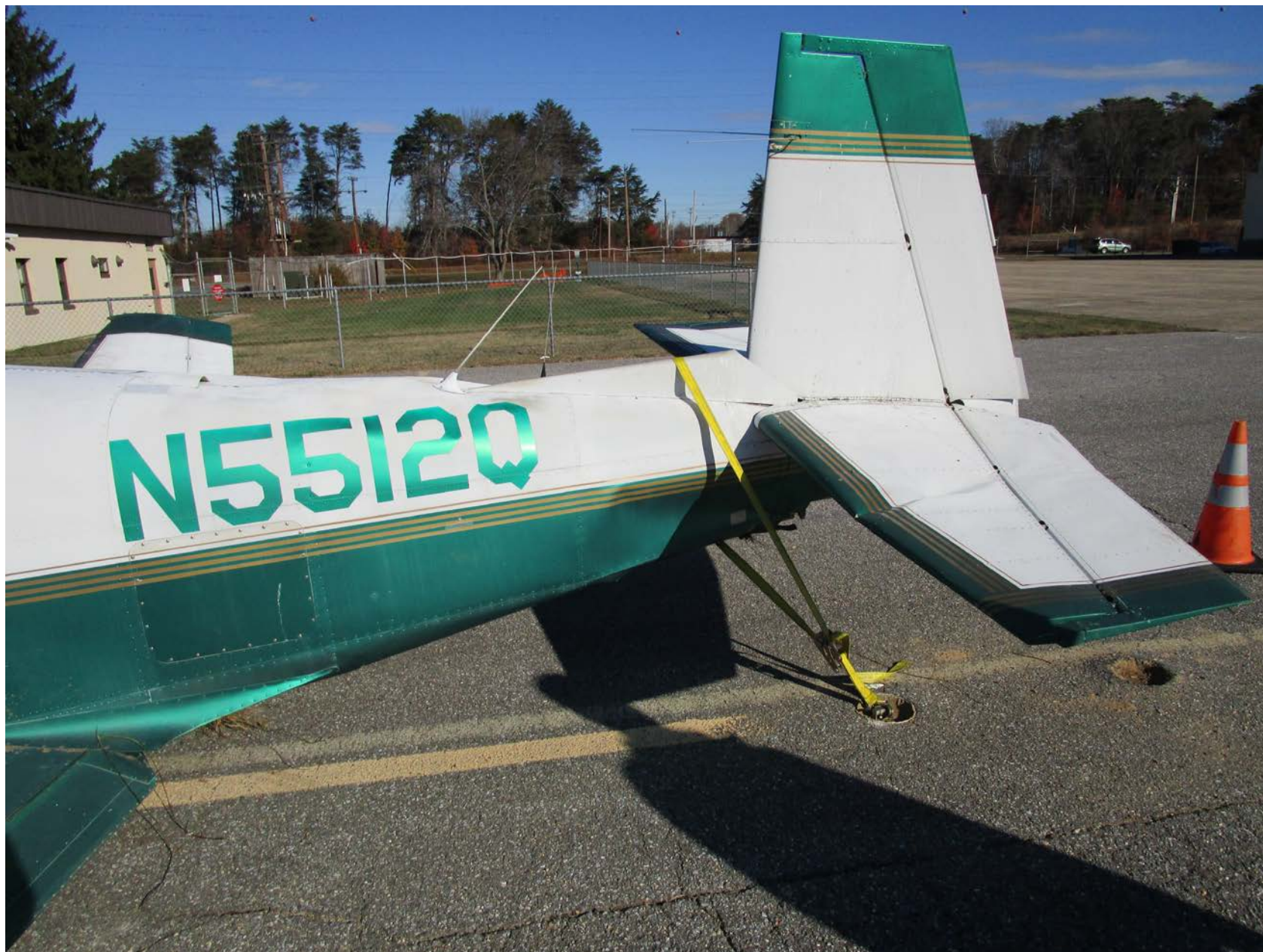
Photo 3 – View of empennage showing buckling on the fuselage and left elevator damage
