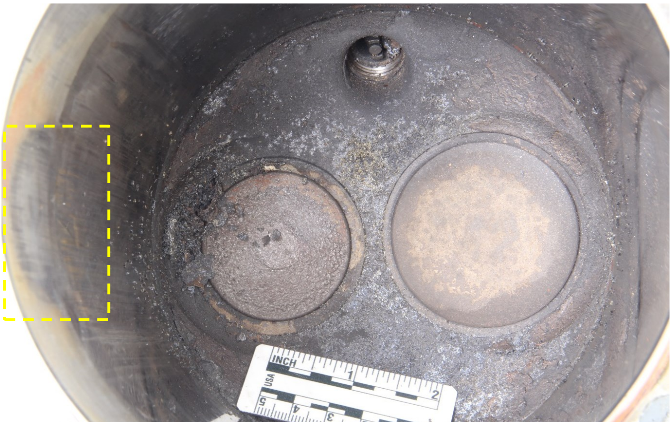
Figure 4 – The inside of the cylinder, as received, showing the deposits near the valves. The area on the left shows indications of corrosion and wear (boxed area).
