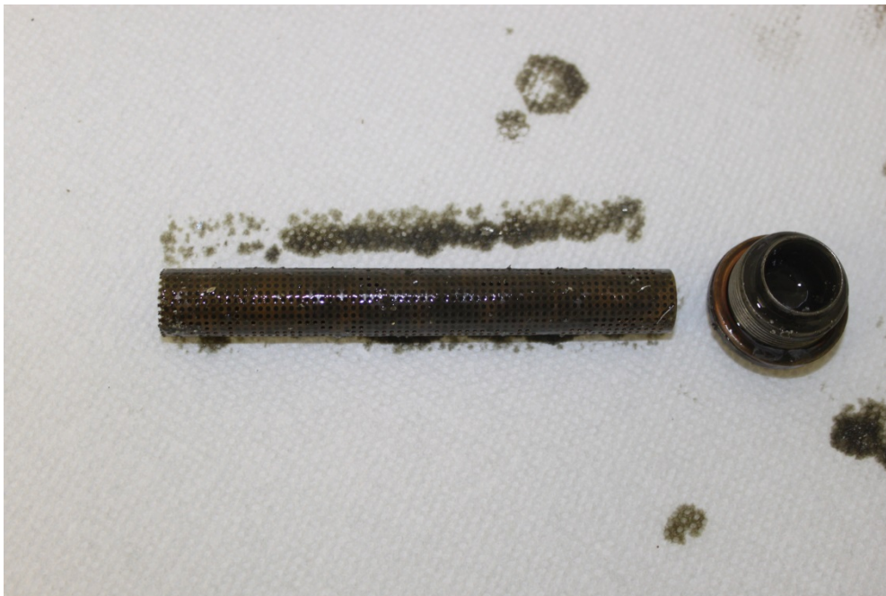
Photo 6. Oil suction screen
