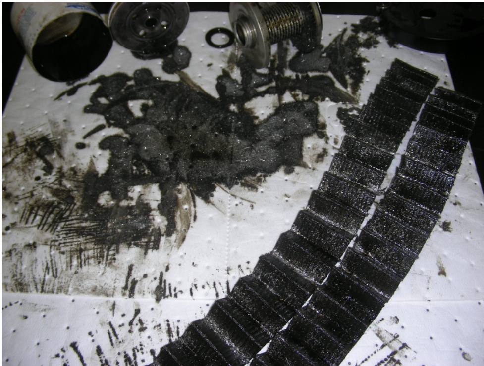
Photo 5. View of disassembled oil filter.
