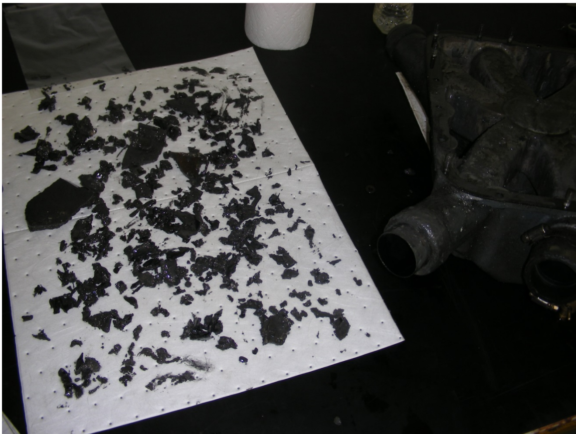
Photo 3. Metallic particles taken out of oil sump
