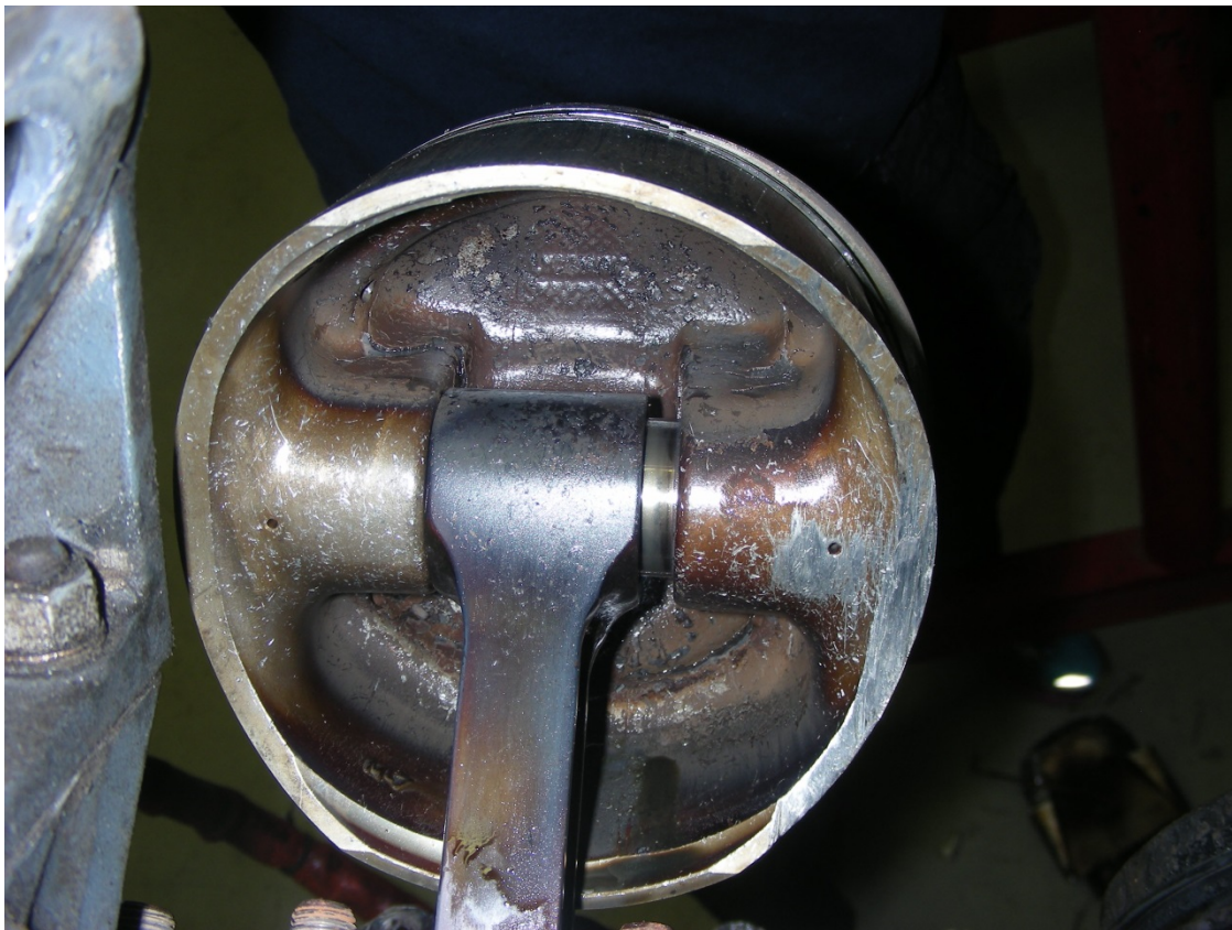
Photo 23. View of Damage on No. 6 Piston
