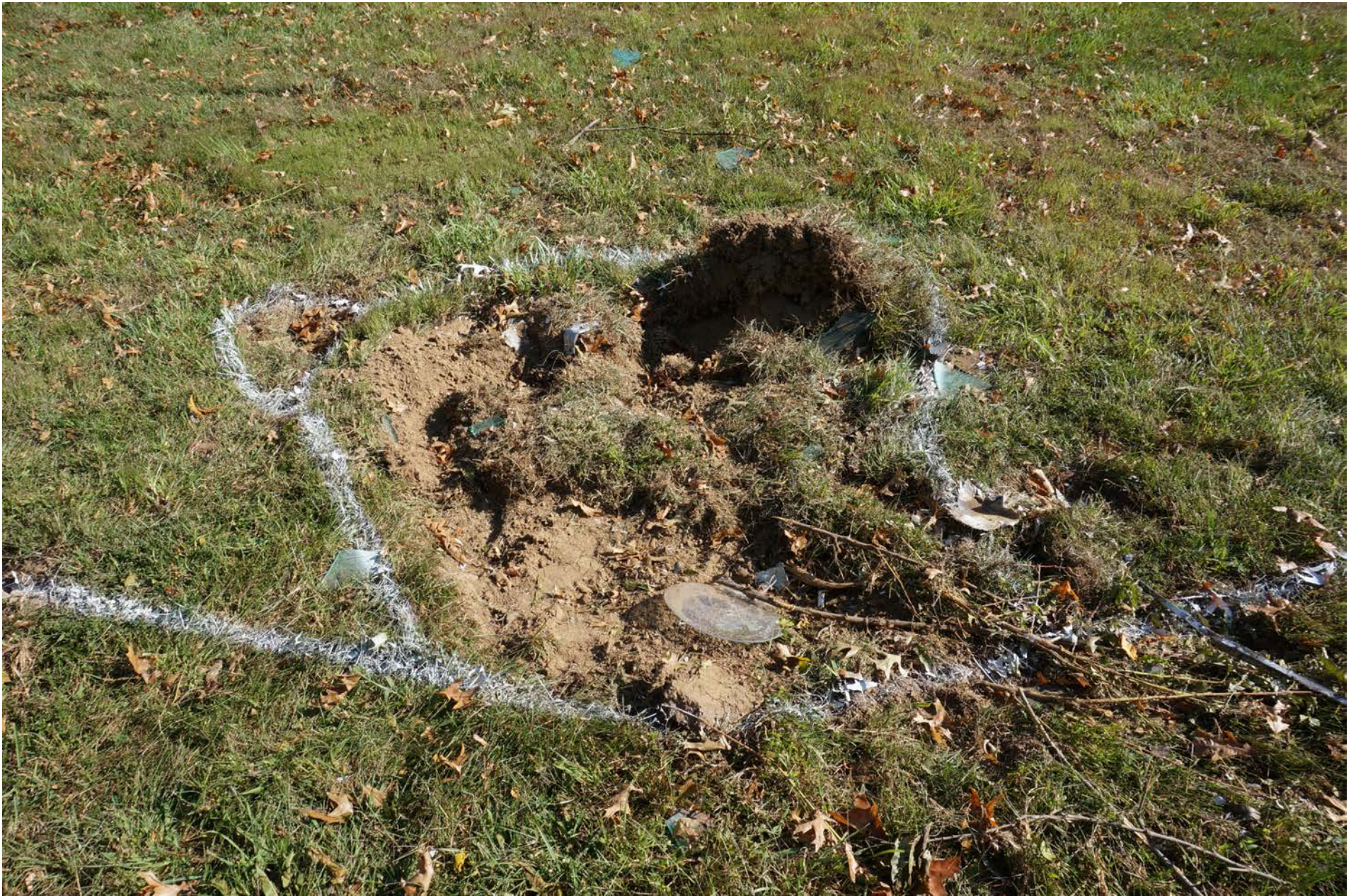
Photo 12 – Initial Impact Point Nose Section Ground Scars – Paint Enhanced
