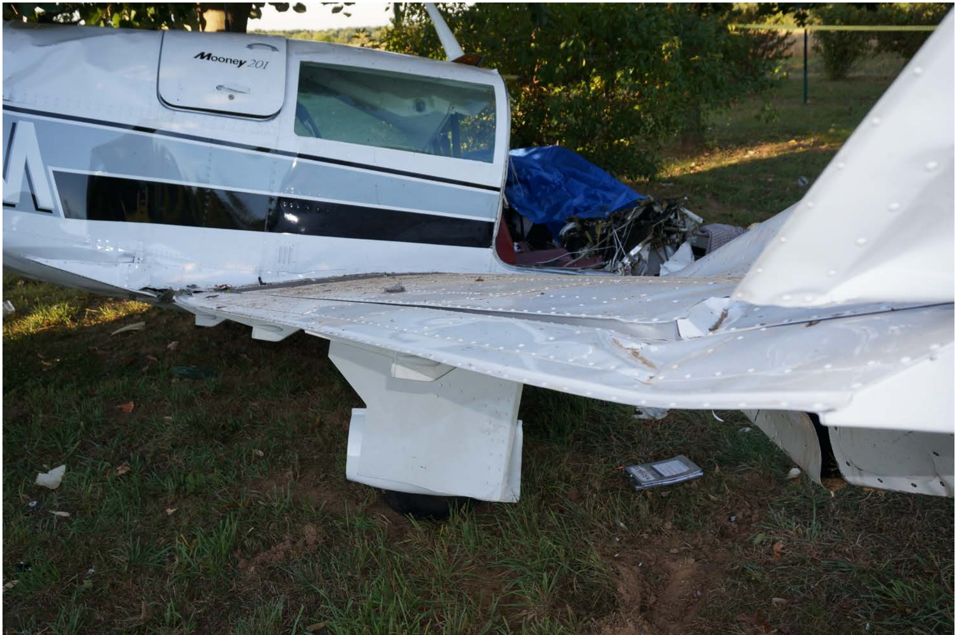
Photo 5 – Right Wing Flap – Retracted Position
