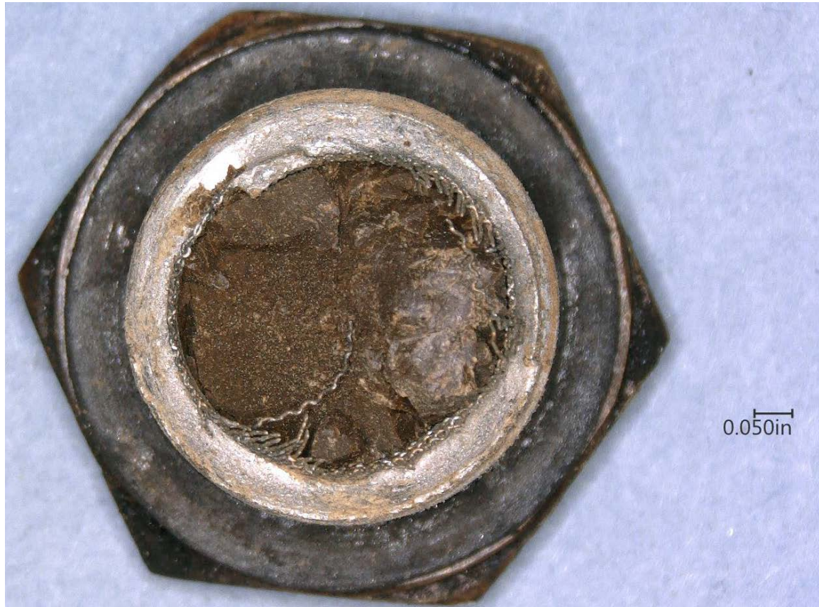
Figure 5. Close-up photograph of underside of fuel screen thumbscrew.
