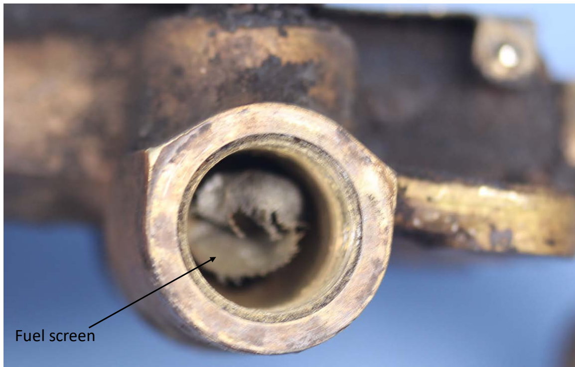
Figure 4. Close-up photograph of torn fuel screen in throttle-body.
