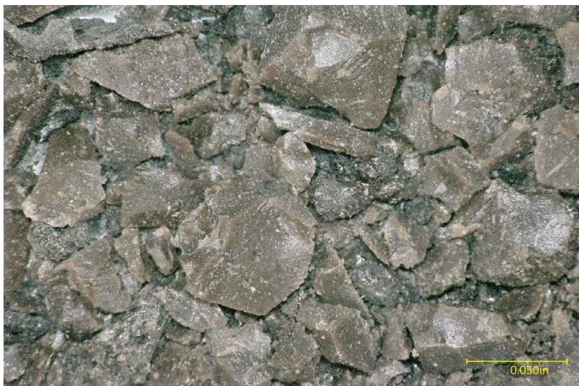
Figure 7. Close-up photograph of debris found in fuel screen.
