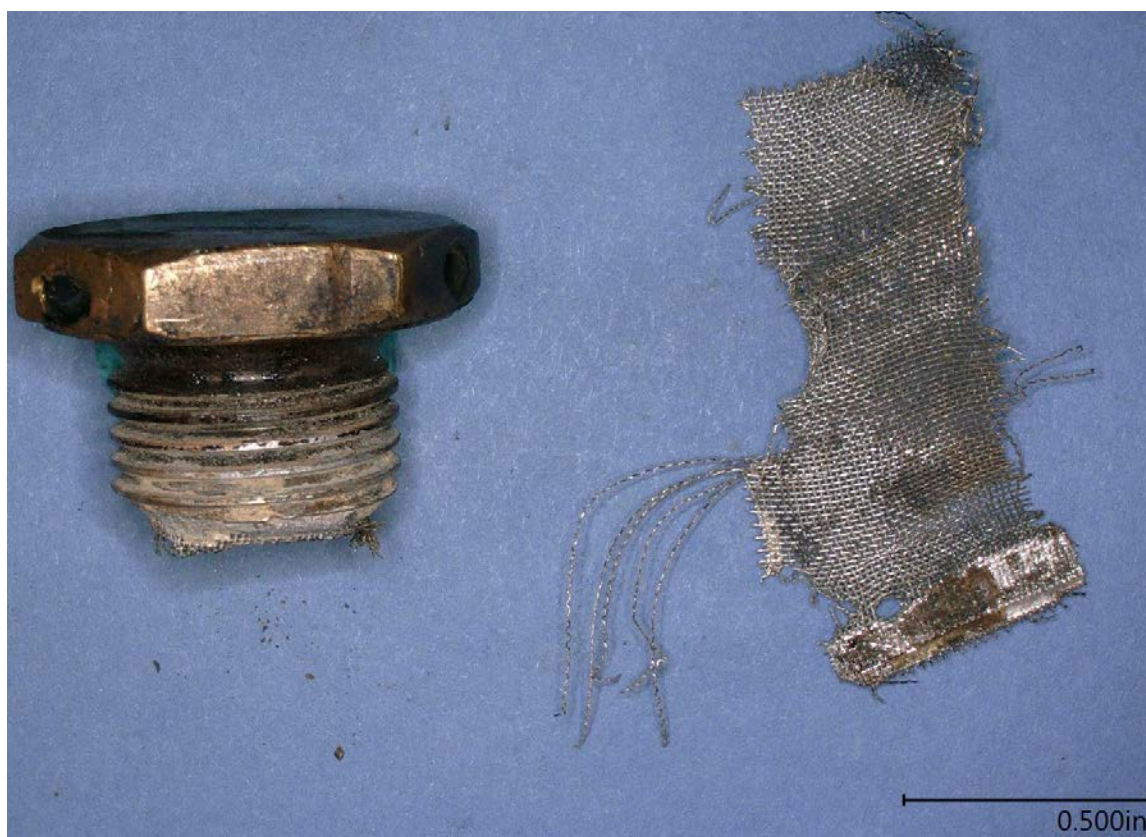
Figure 6. Photograph of thumbscrew and remnants of fuel screen.
