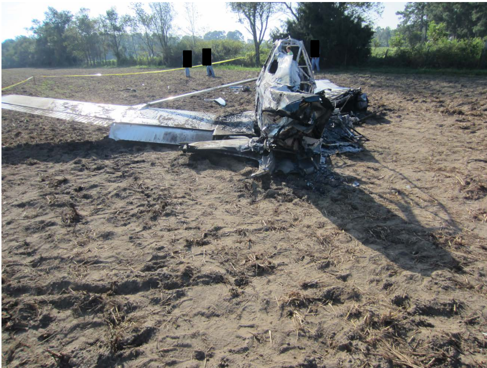
Photo 3 – View of Empennage Folded Under Fuselage
