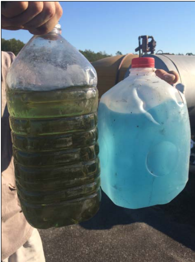
Photo 1: Fuel samples pumped from the pilot's trailer-based fuel supply.
