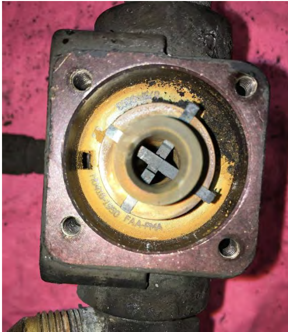
Picture 7. View of Rotor and Vanes inside the Right Engine Driven Fuel Pump
