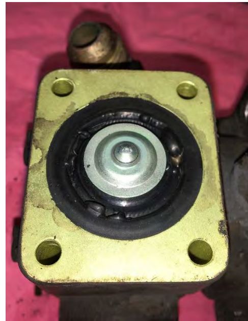
Picture 5. View of heat damaged relief valve diaphragm.
