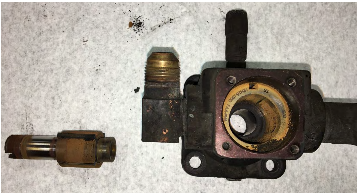
Picture 9. View of rotor and vanes removed from pump liner.
