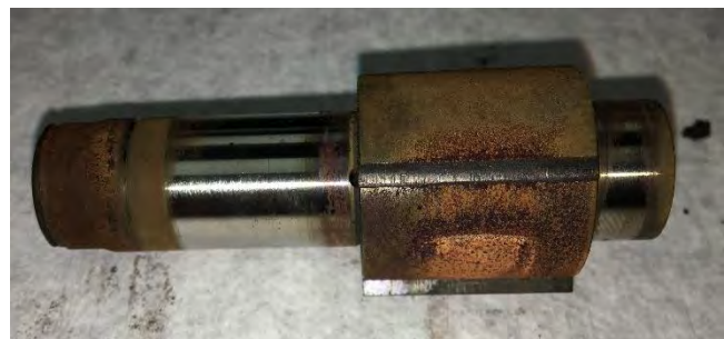
Picture 8. View of Rotor and Vanes Removed from Housing.
