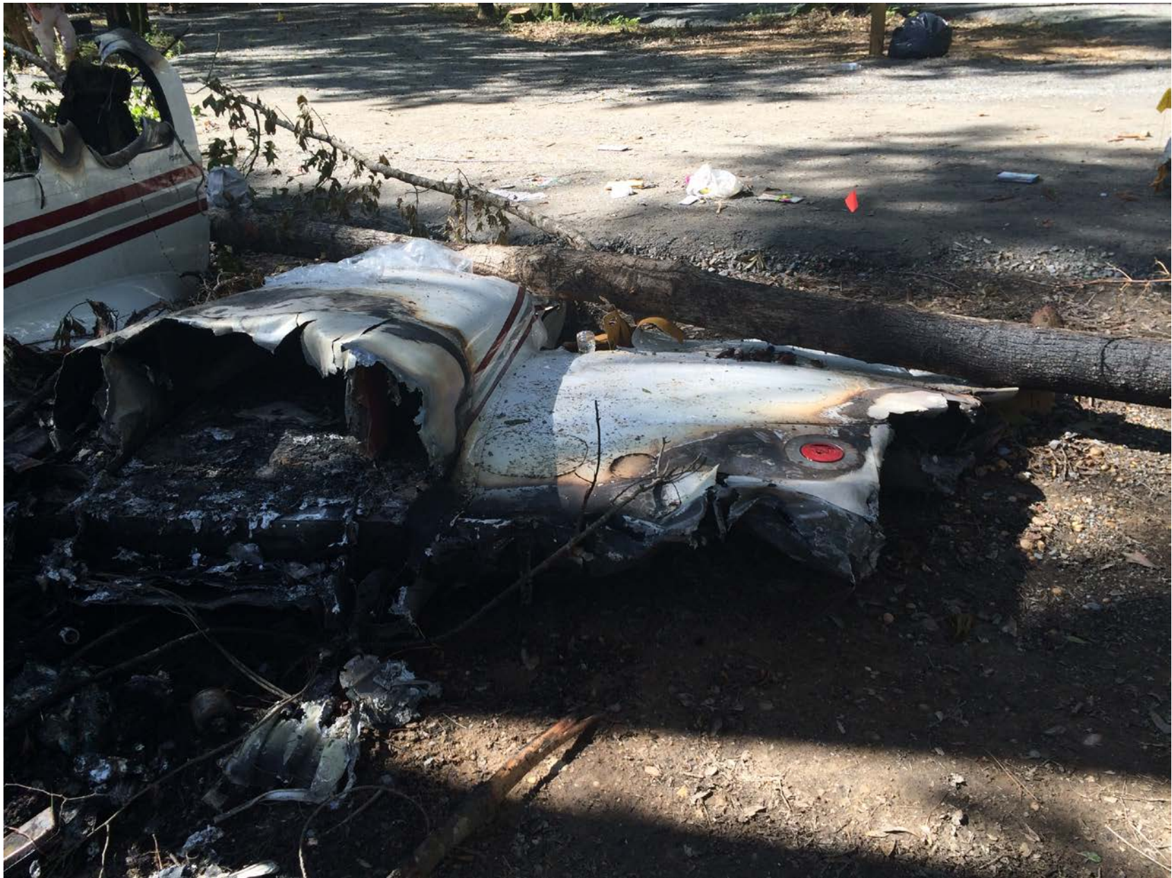
Photo 6 – View of Left Inboard Section of Wing
