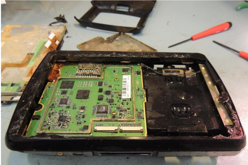
Figure 1. Garmin Aera 796 GPS, with damaged display panel removed.
