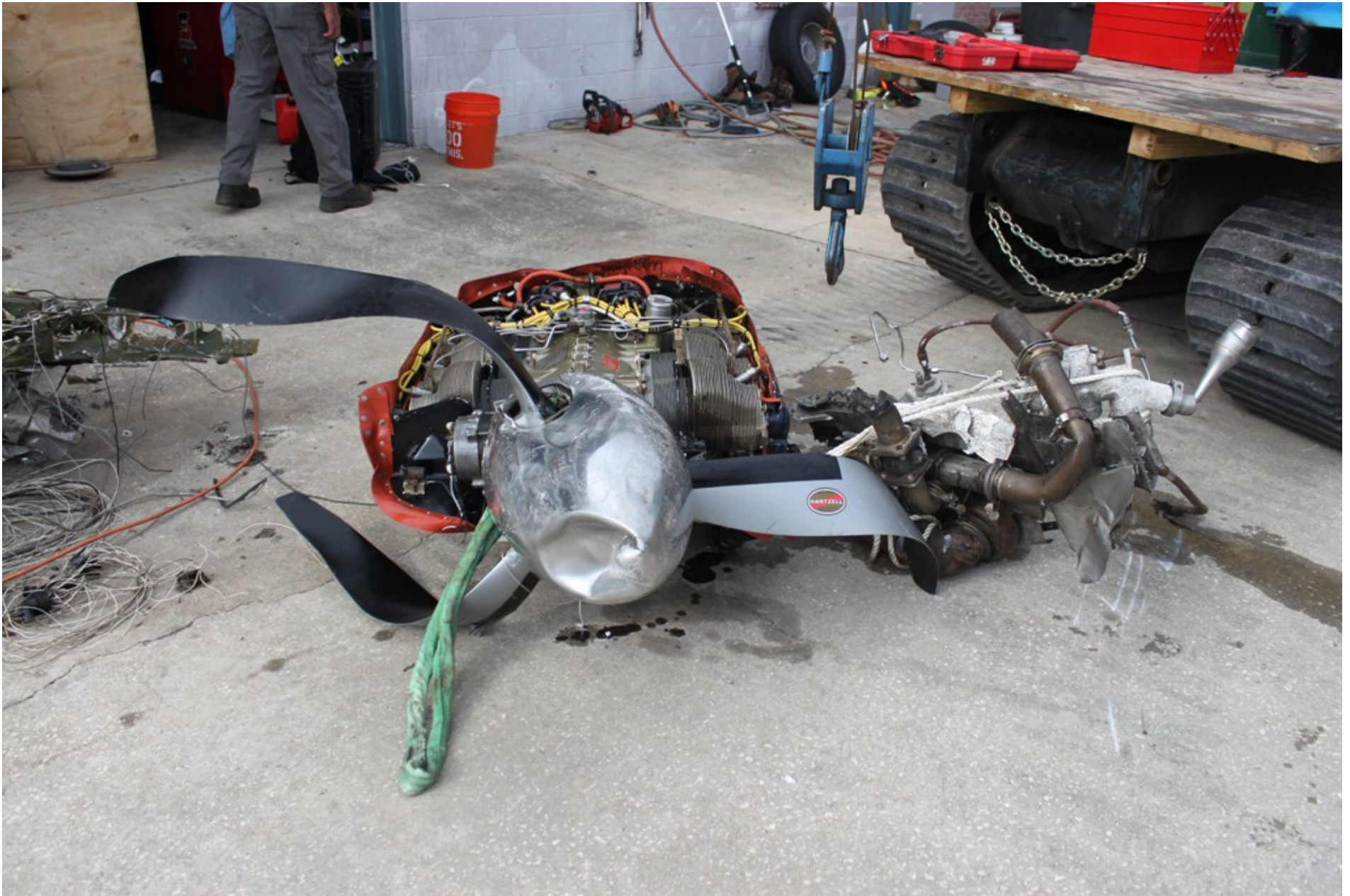
Photo 11 - NTSB Digital Photograph. View Showing the Right Propeller and Portion of Separated Right Engine, and Right Engine Components.
