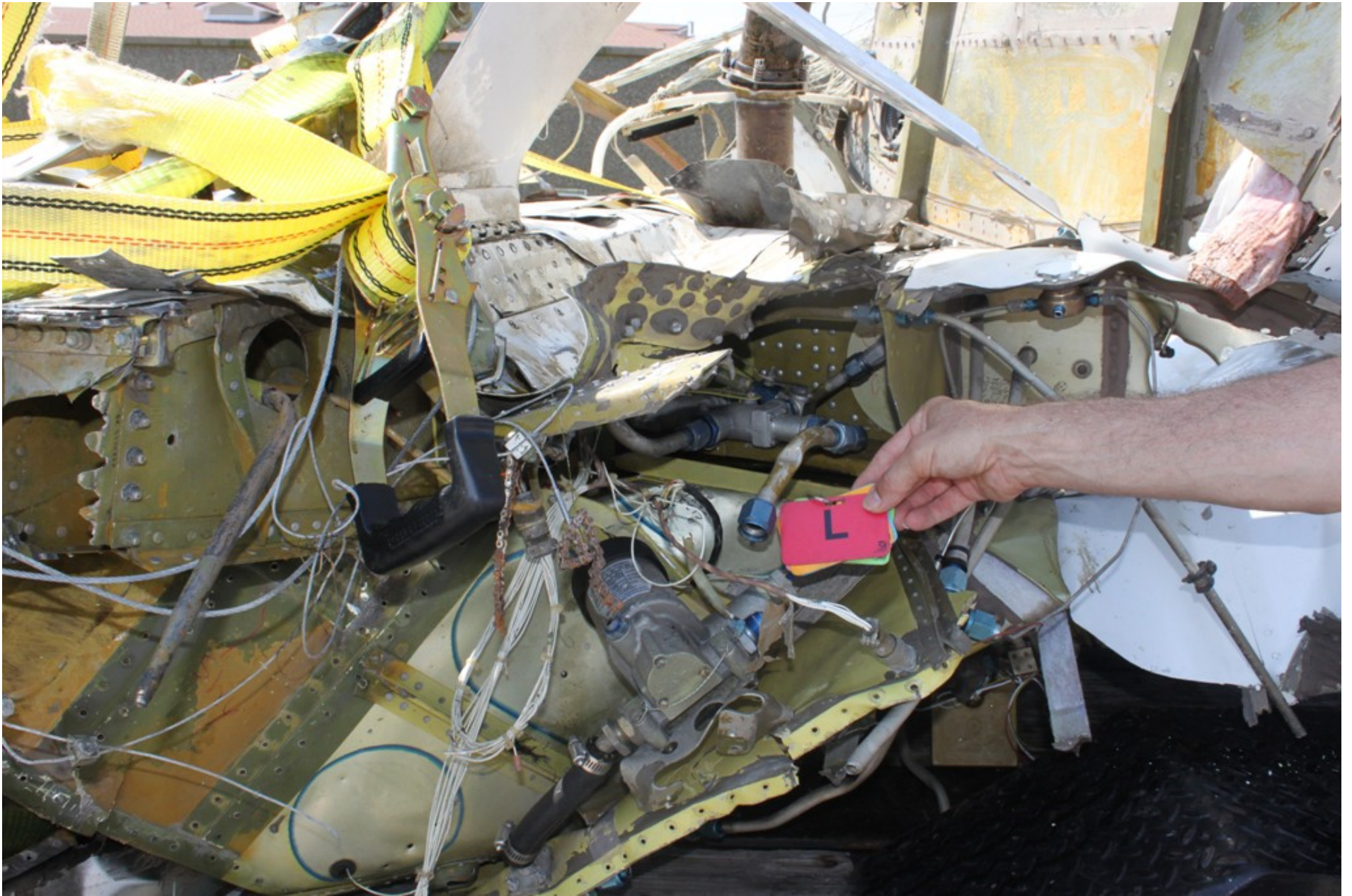
Photo 6 - NTSB Digital Photograph. View Showing the Separated Outlet Fuel Line from the Left Auxiliary Fuel Pump.
