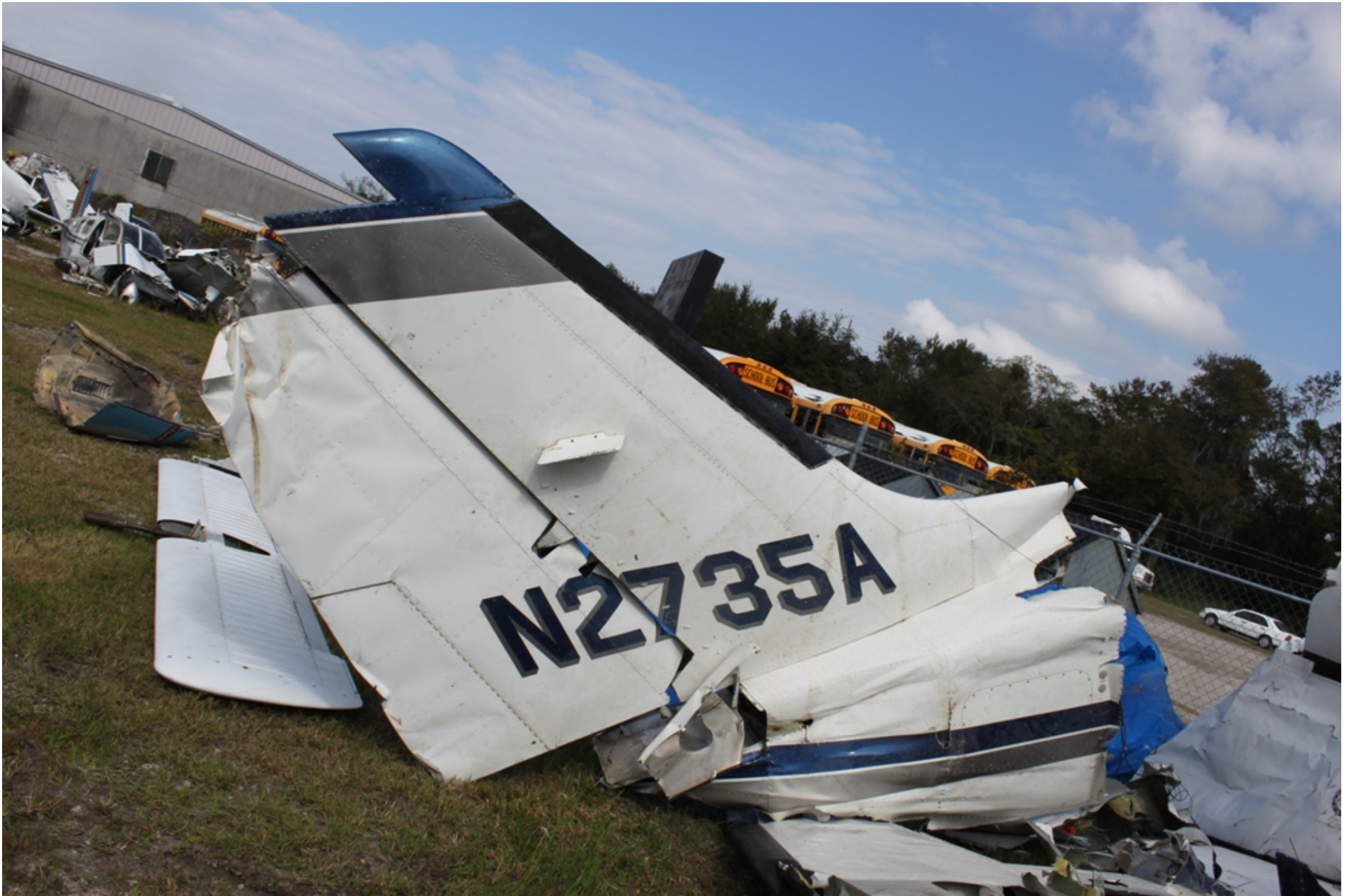
Photo 13 - NTSB Digital Photograph. View Showing the Right Side of the Vertical Stabilizer, Rudder, Rudder Trim Tab, and Portion of Empennage.
