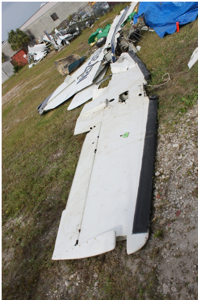
Photo 14 - NTSB Digital Photograph. View Showing the Horizontal Stabilizer with Attached Elevators.
