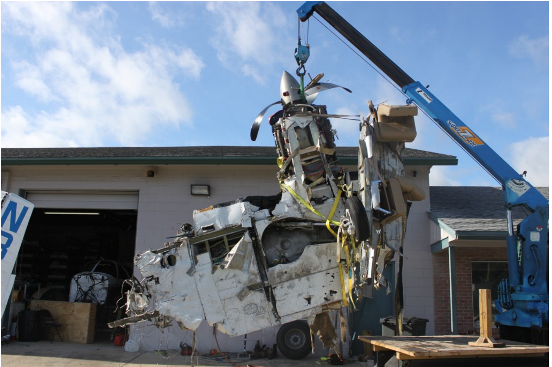
Photo 5 - NTSB Digital Photograph. View of the Bottom Portion of the Left Wing, Left Engine and Propeller.
