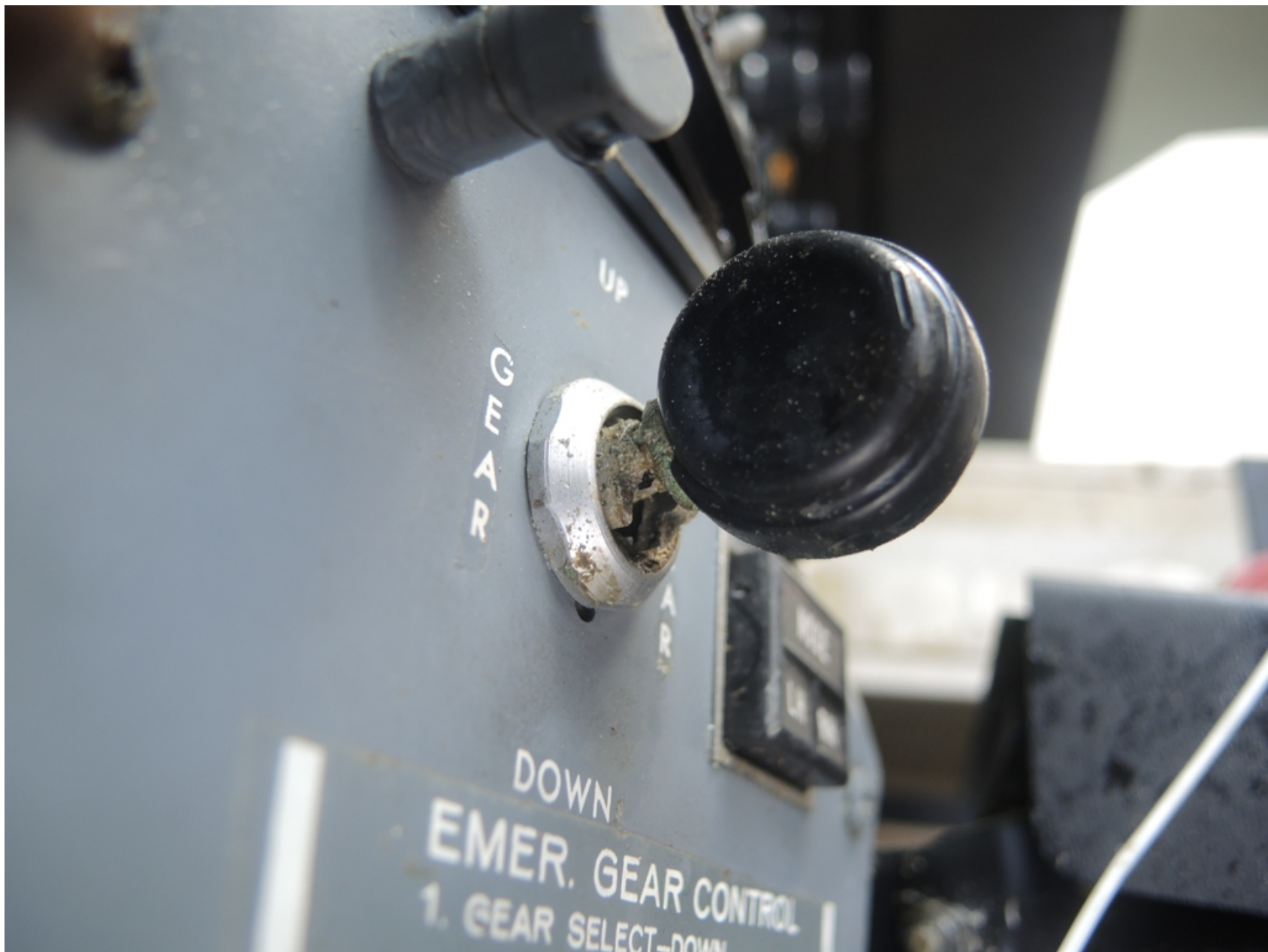
Photo 9 – Textron Aviation Digital Photograph. View Showing the Position of the Landing Gear Selector.
