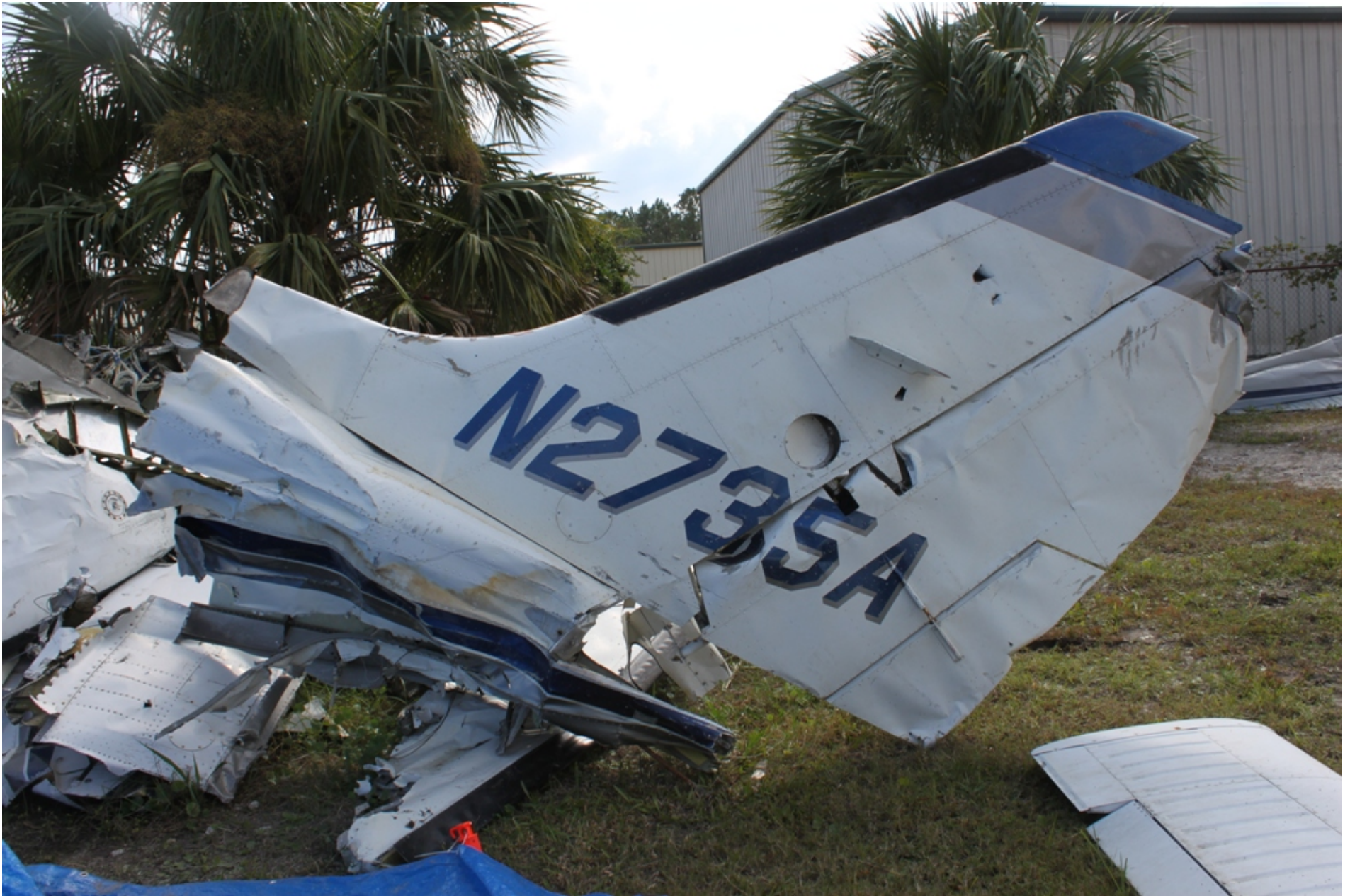
Photo 12 - NTSB Digital Photograph. View Showing the Left Side of the Vertical Stabilizer, Rudder, Rudder Trim Tab, and Portion of Empennage.
