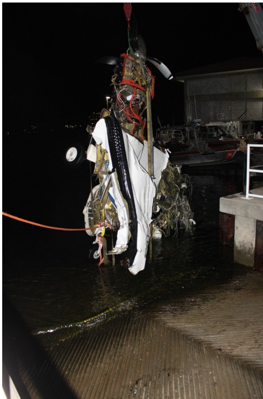
Photo 3 - NTSB Digital Photograph. View of the Left Engine and Propeller, and Portion of Left Wing During Recovery
