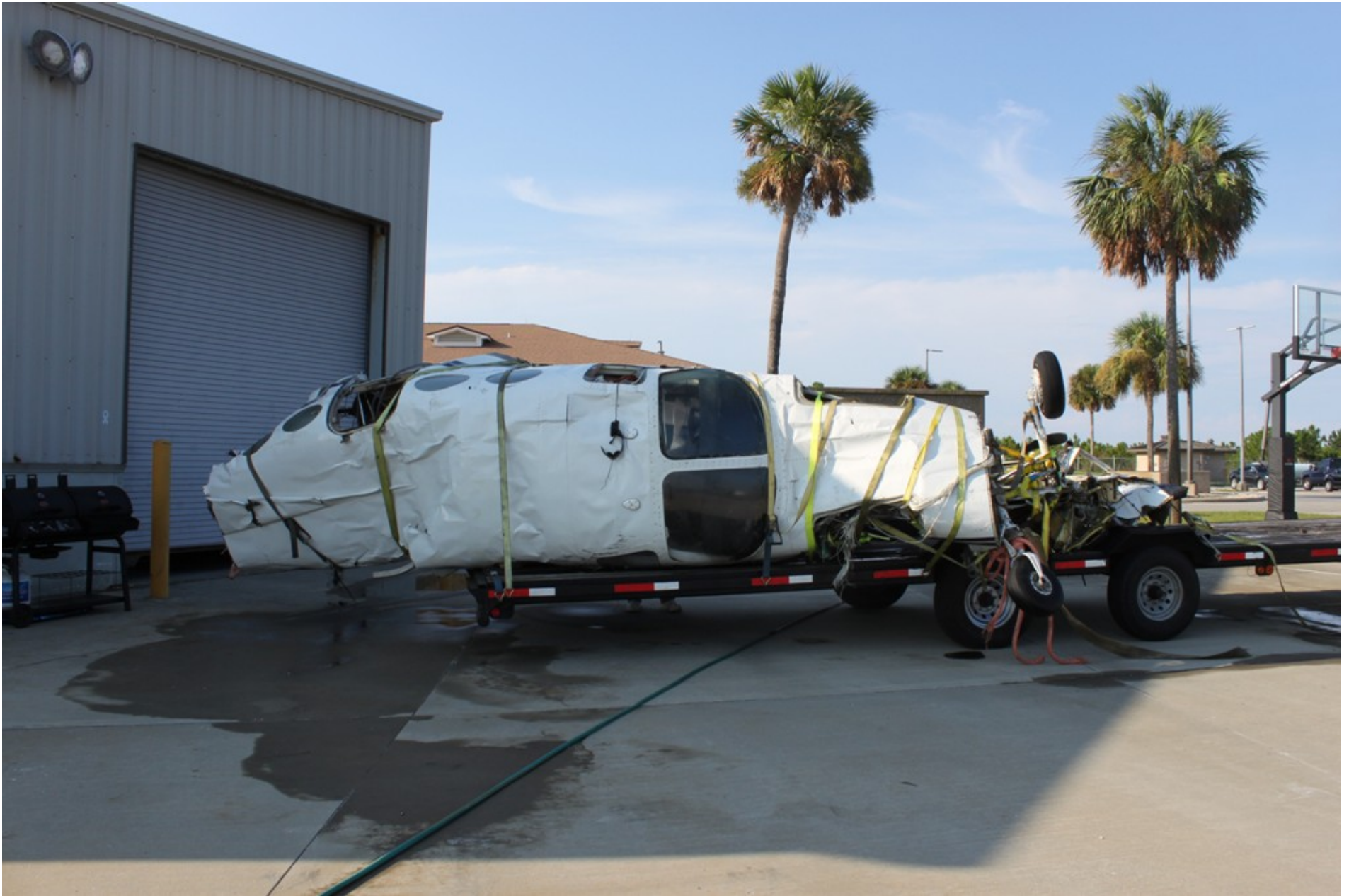
Photo 1 – NTSB Digital Photograph. View of the Upper Side of the Fuselage Following Recovery from the Gulf of Mexico
