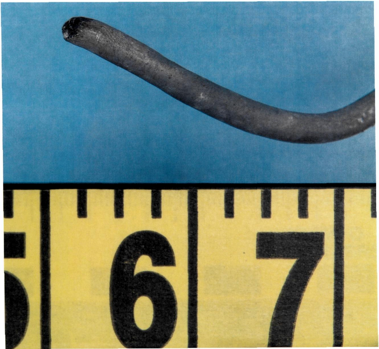
Figure 16. Closeup of second small outlet on fuel pump.
