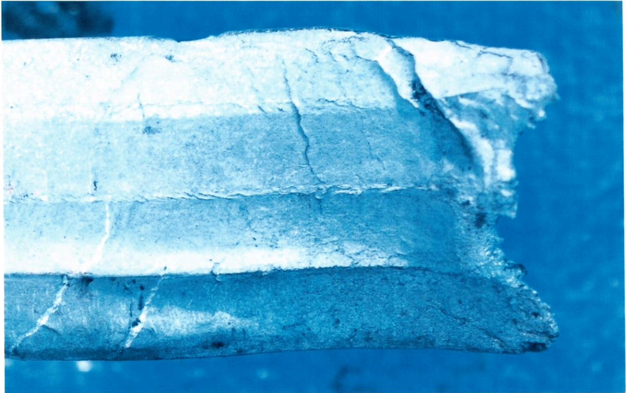
Figure 6. Closeup photograph of broomstrawed end.
