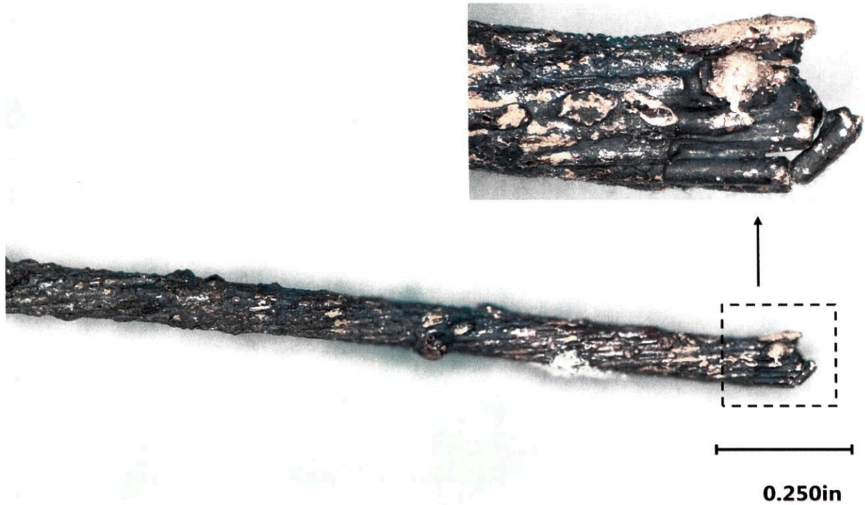
Figure 12. Closeup photograph of arcing, beading and melting damage to end of power wiring section.
