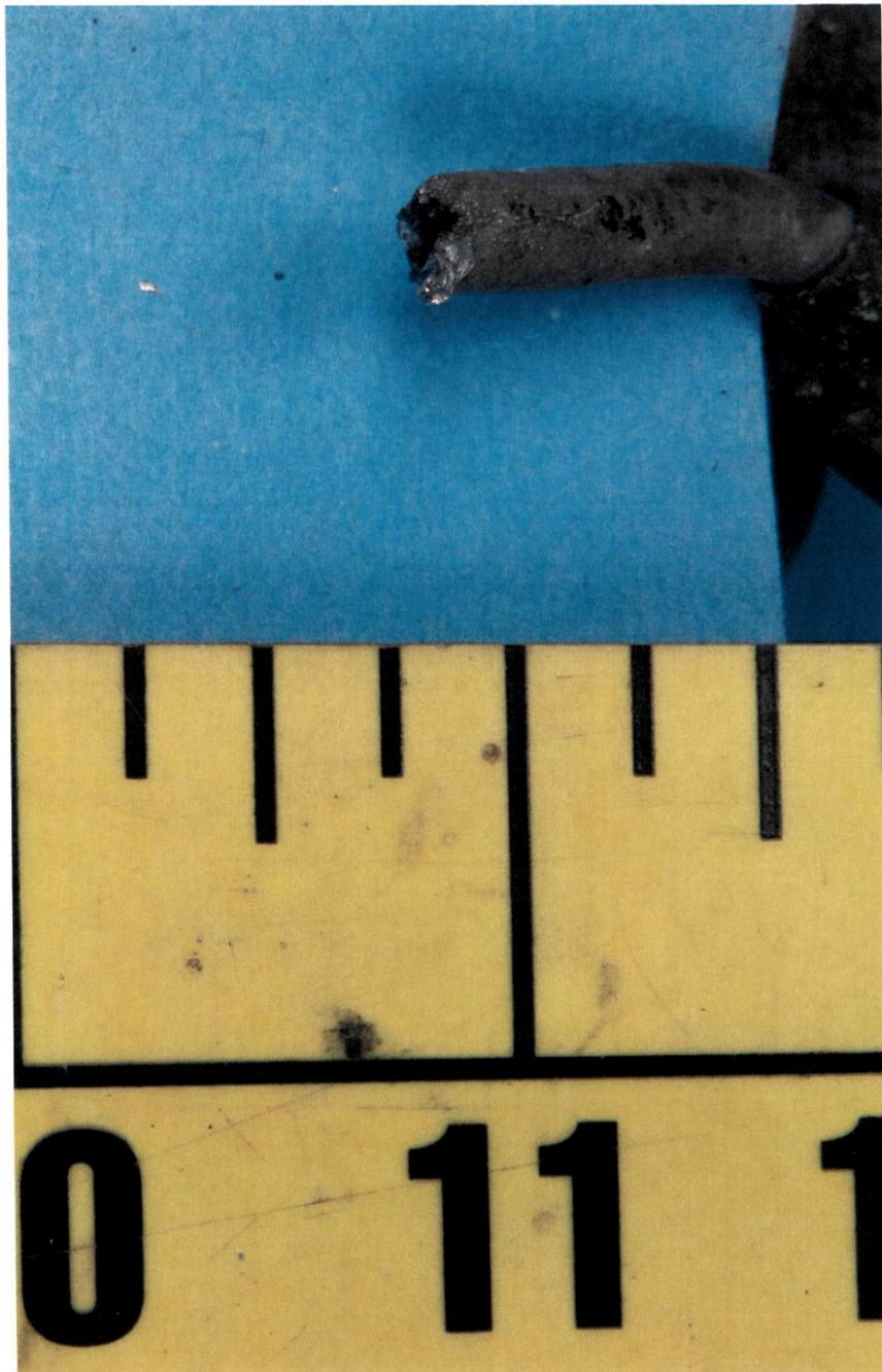
Figure 15. Closeup of one small outlet on fuel pump.
