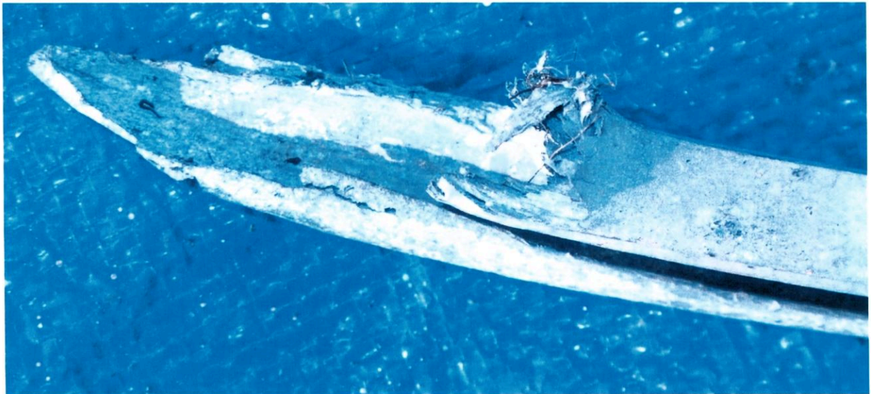
Figure 5. Closeup photograph of one of broomstrawed end.
