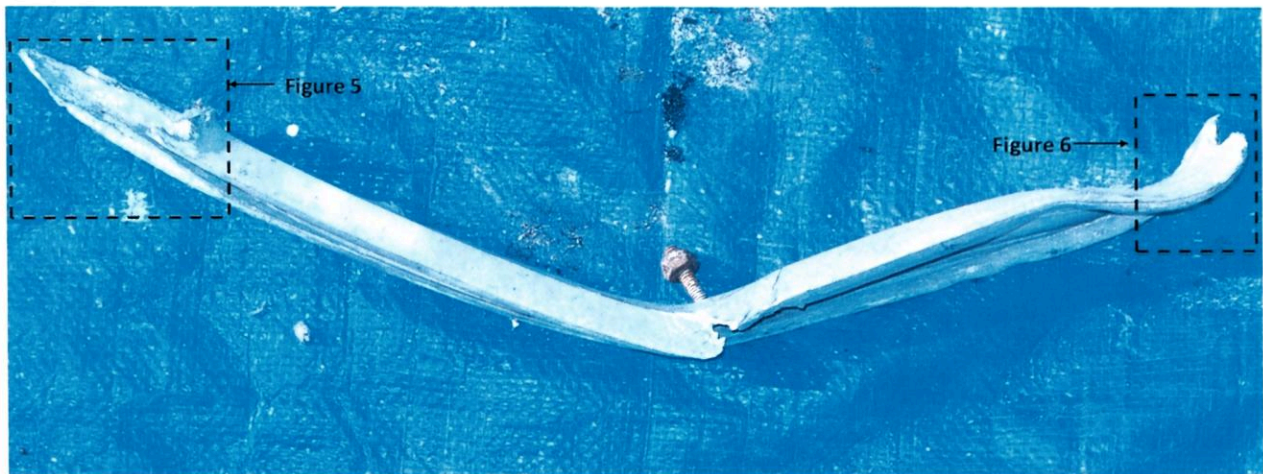
Figure 4. Section of aircraft structure with broomstrawed ends.
