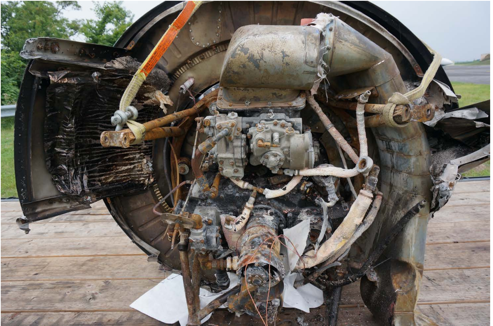
Photo 17 – Fire Sleeved Hoses
