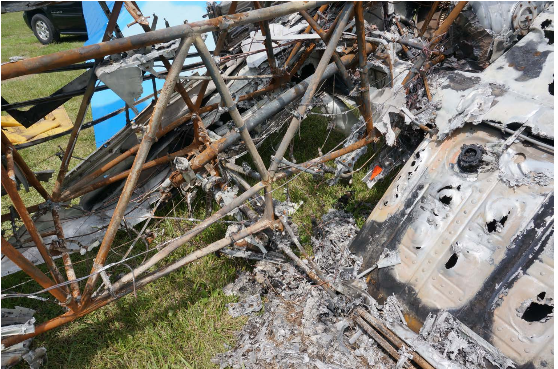
Photo 13 – Area of Fire Origin
