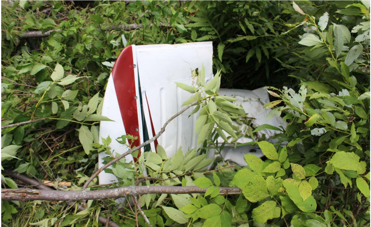
Figure 2 Portion of the right side of the horizontal stabilator along the debris path.
