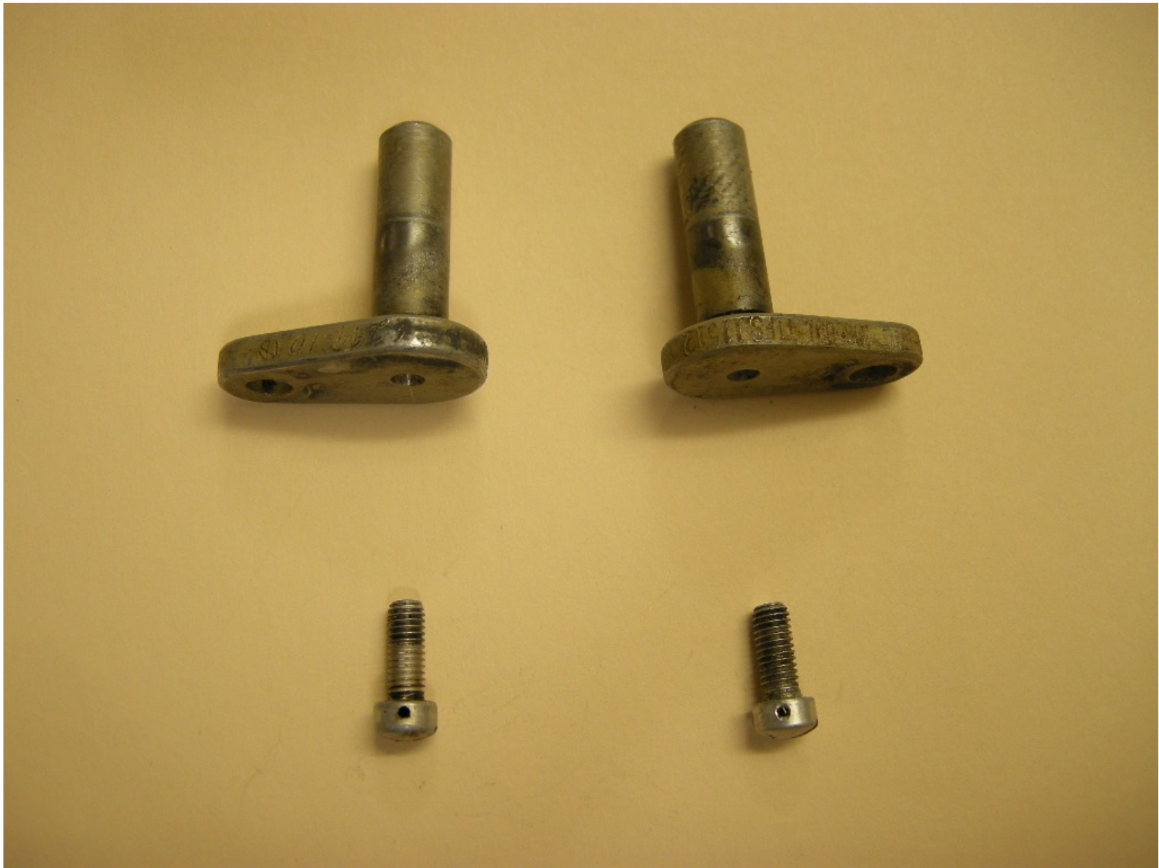
Photo 12 – Collective Lever Pins and Attaching Screws (NTSB Photo)
