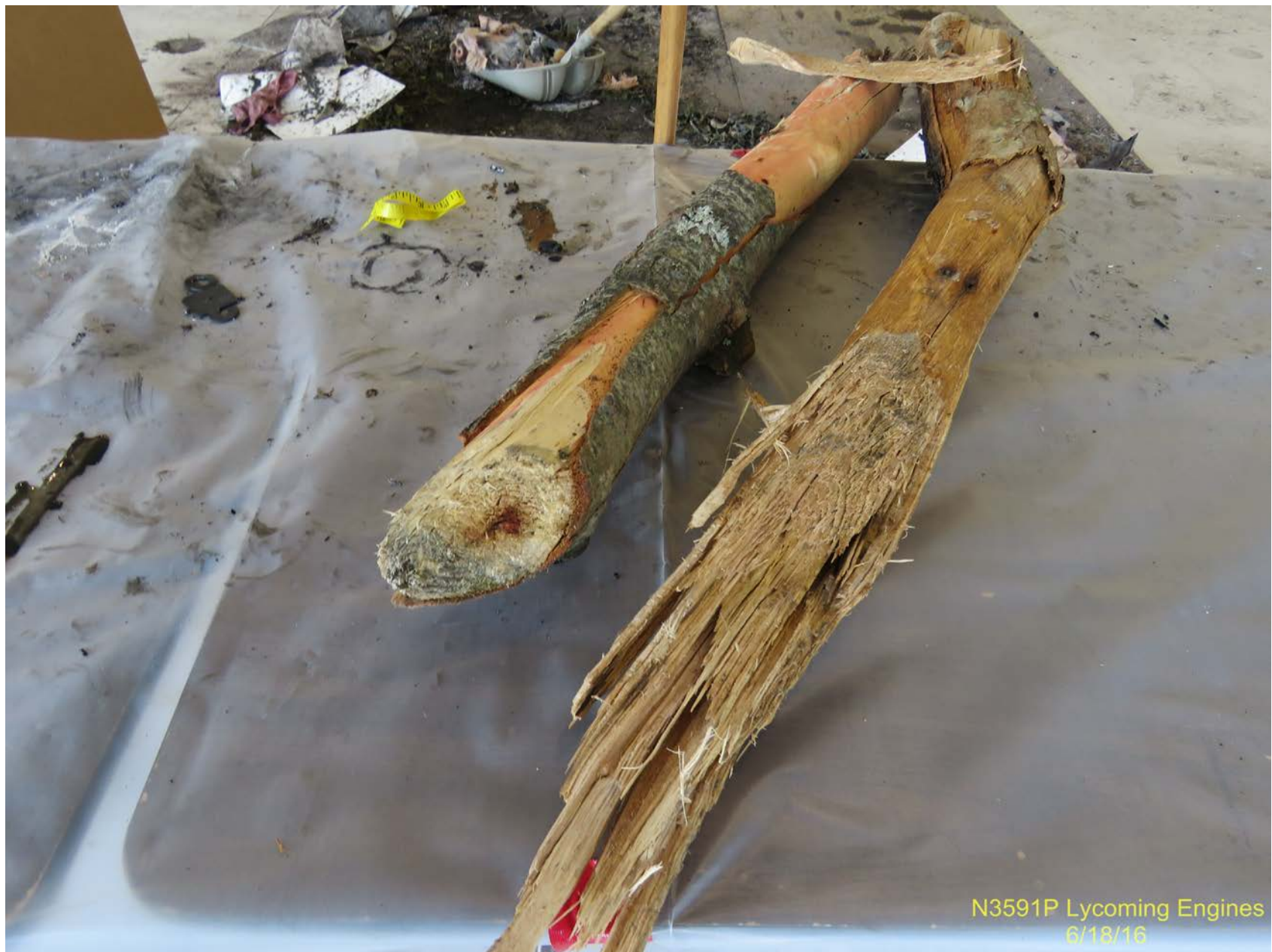
Photo 6 – View of Angularly Cut Wood Recovered from Crash Site (Lycoming)
