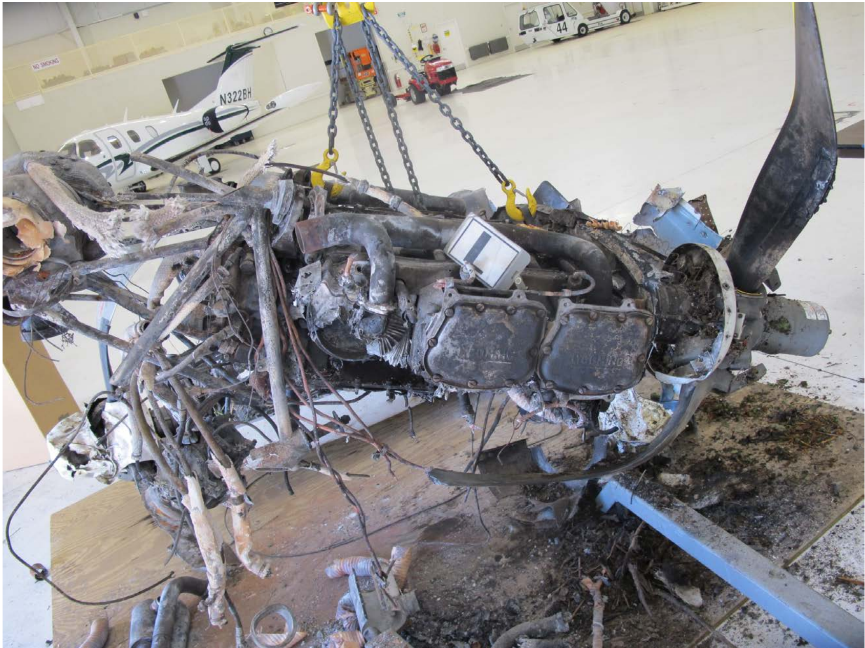
Photo 4 – View of Left Engine After Recovery (Lycoming)
