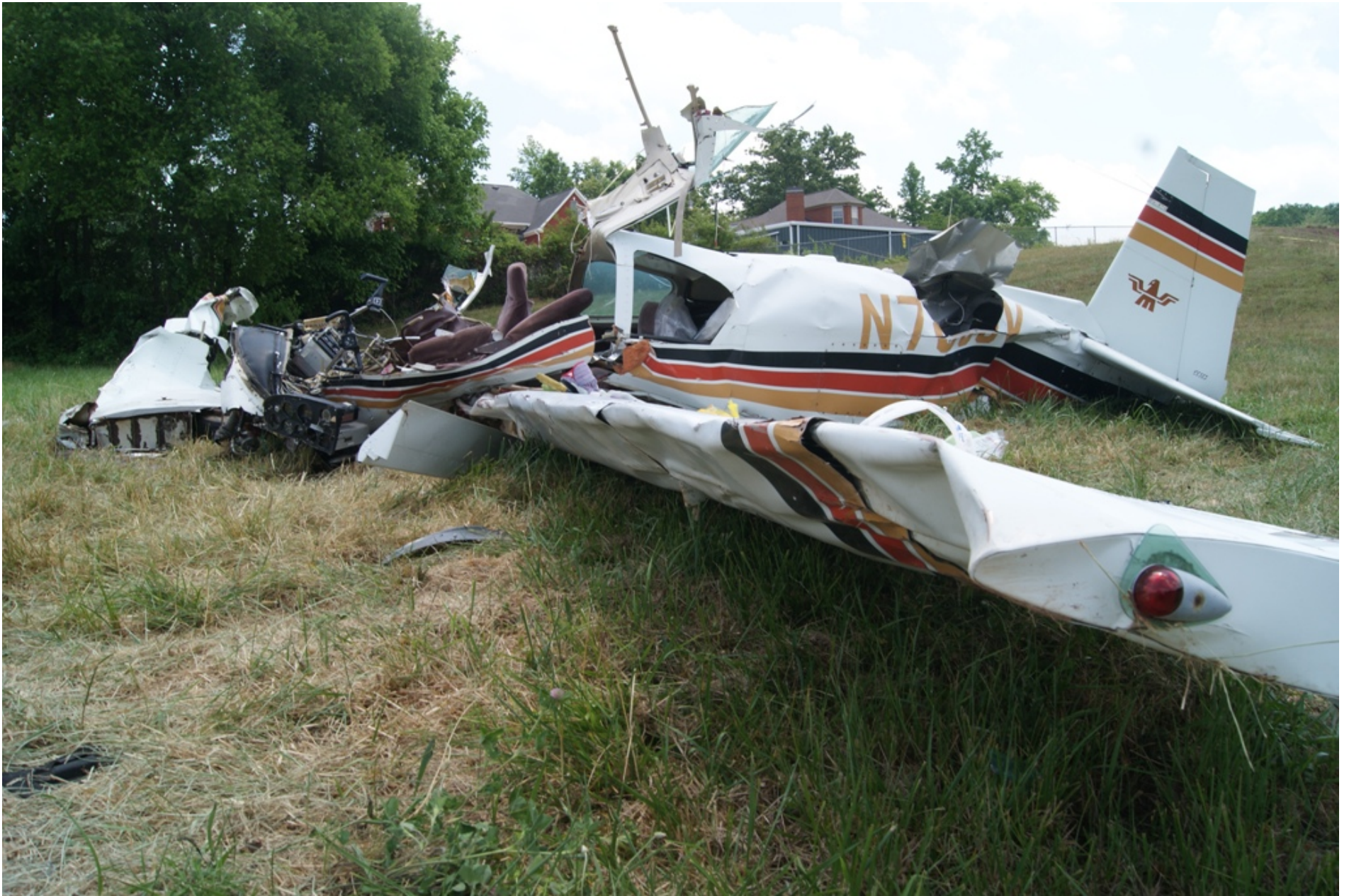
Photo 4 – Close-up View of Left Wing Damage
