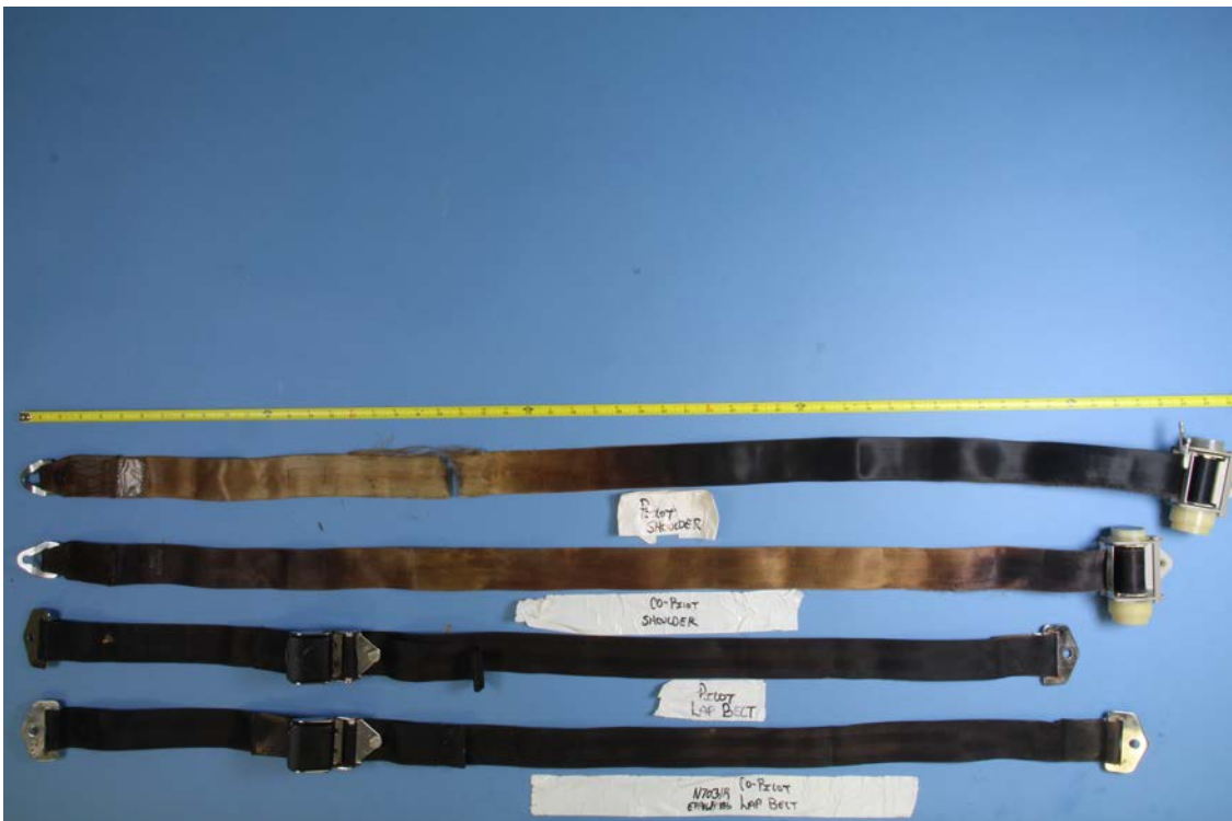
Photo 8. Lapbelts and shoulder harnesses of both restraints.
