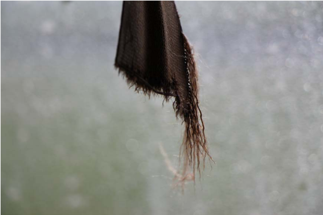
Photo 7. Close-up of frayed end of pilot's shoulder harness.
