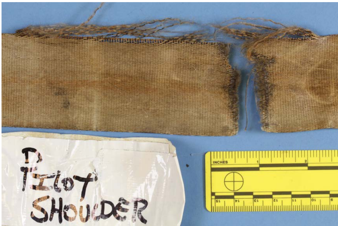
Photo 9. Area of fraying and separation of the pilot's shoulder harness.
