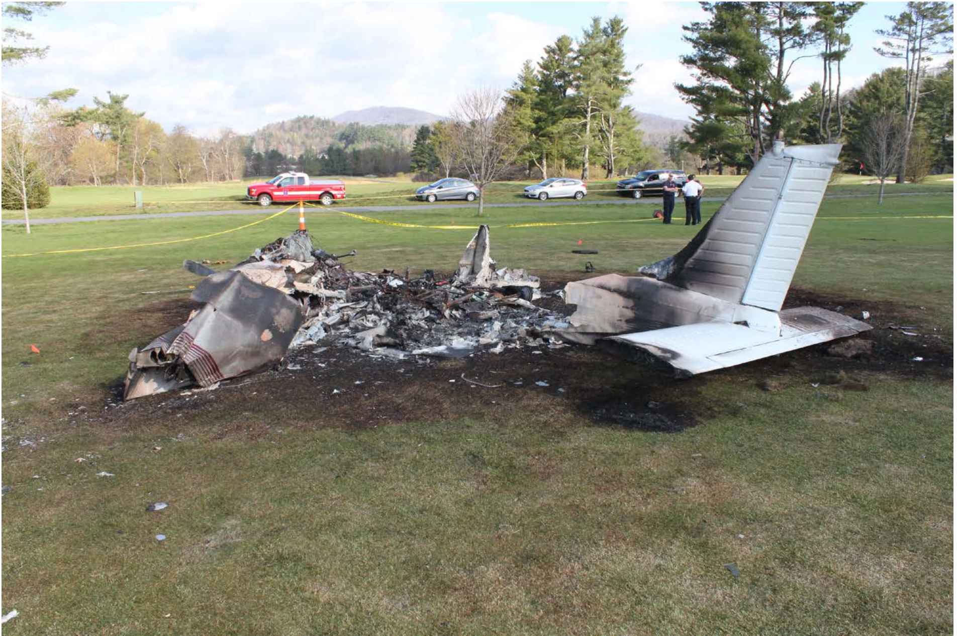
Photo 3 – View from rear of airplane showing fire damage
