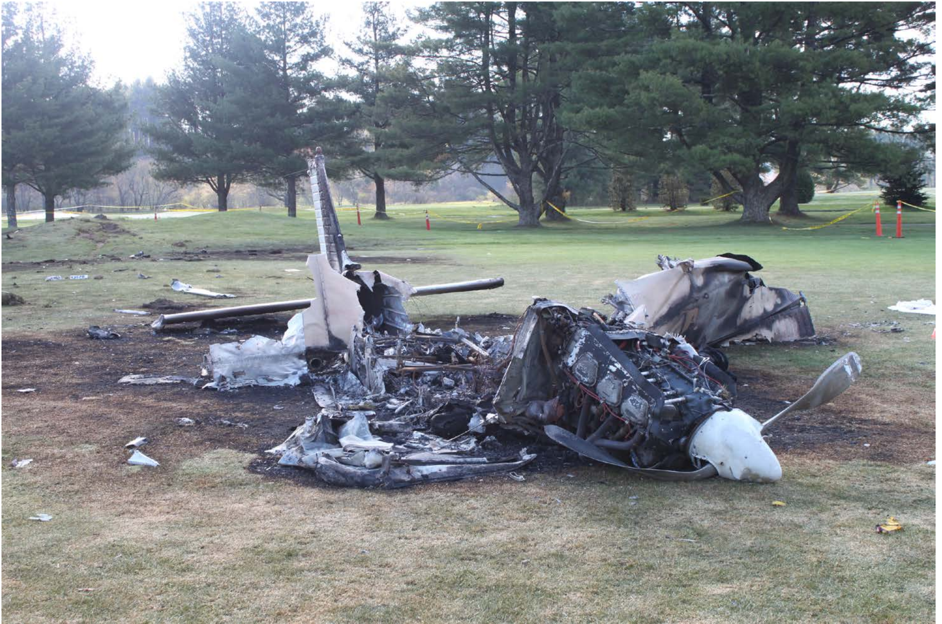
Photo 1 – View of front of airplane from right side showing fire damage
