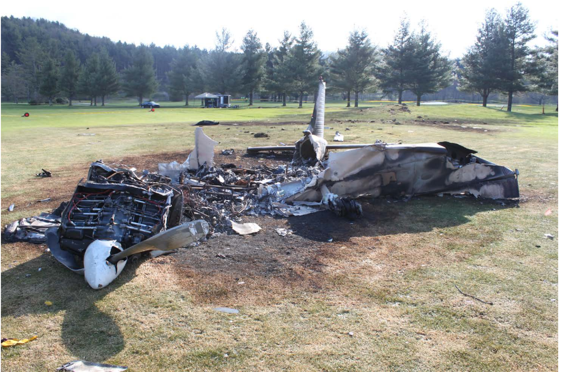
Photo 2 – View of front of airplane from left side showing fire damage
