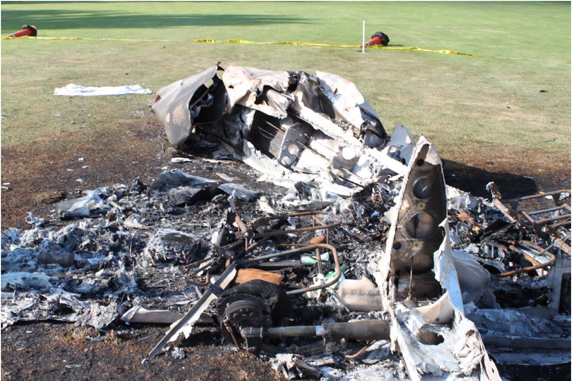
Photo 4 – View of cabin section fire damaged
