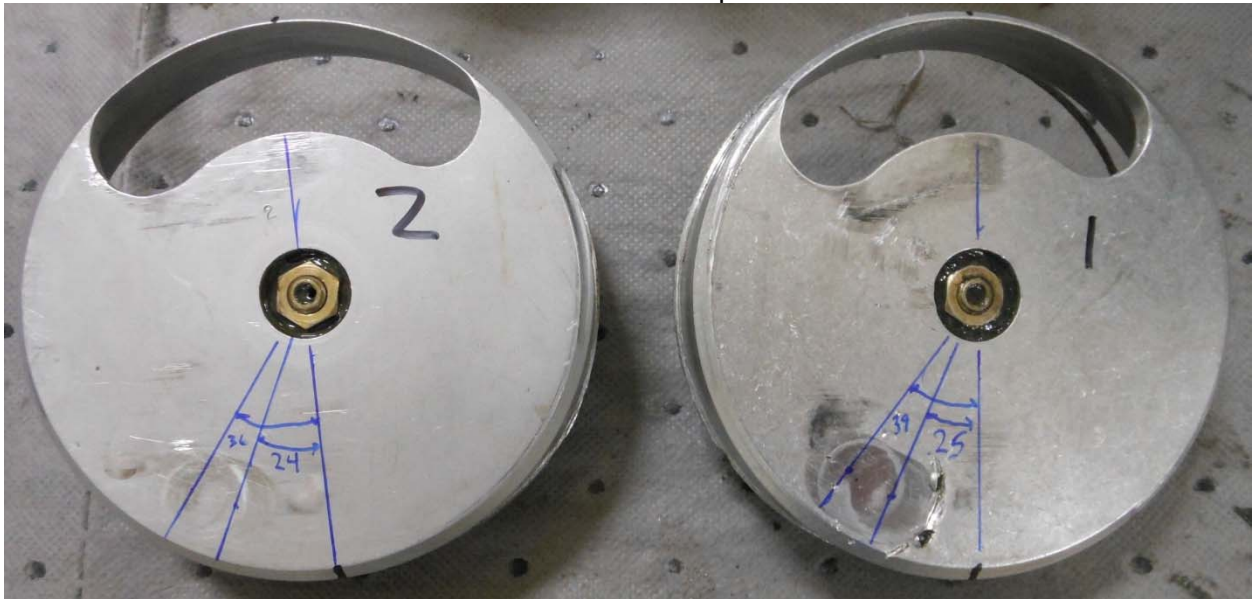
Photo #7 – Preload plates
