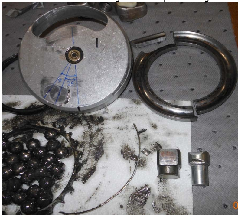
Photo #8 – Blade #1 bearing races and pitch change knob
