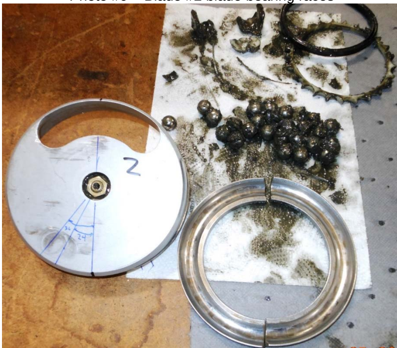
Photo #9 – Blade #2 blade bearing races
