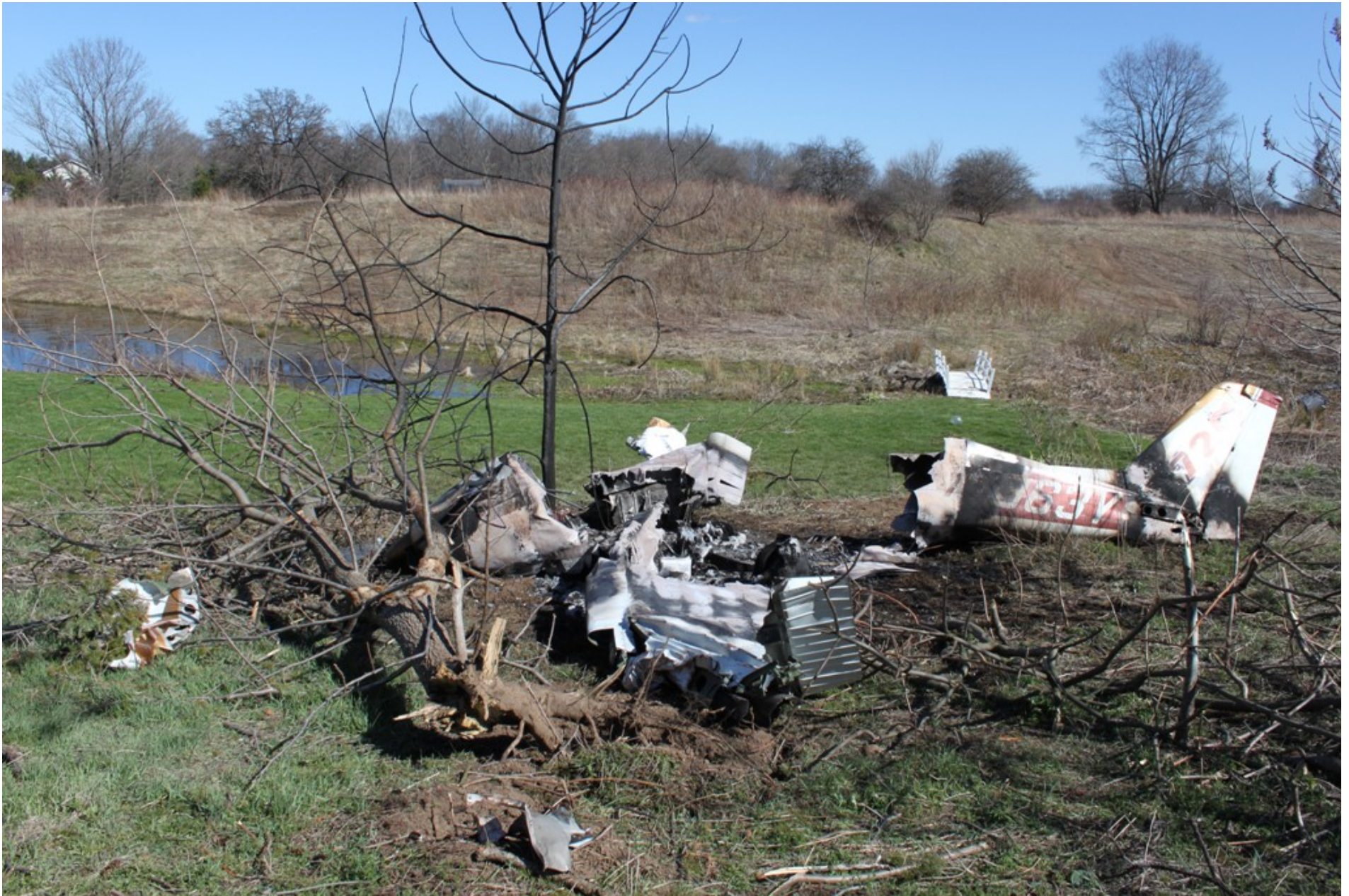
Photo 8 – NTSB Digital Photograph. Left Side View of the Wreckage. Note the Extensive Fire Damage to the Cockpit and Fuselage.
