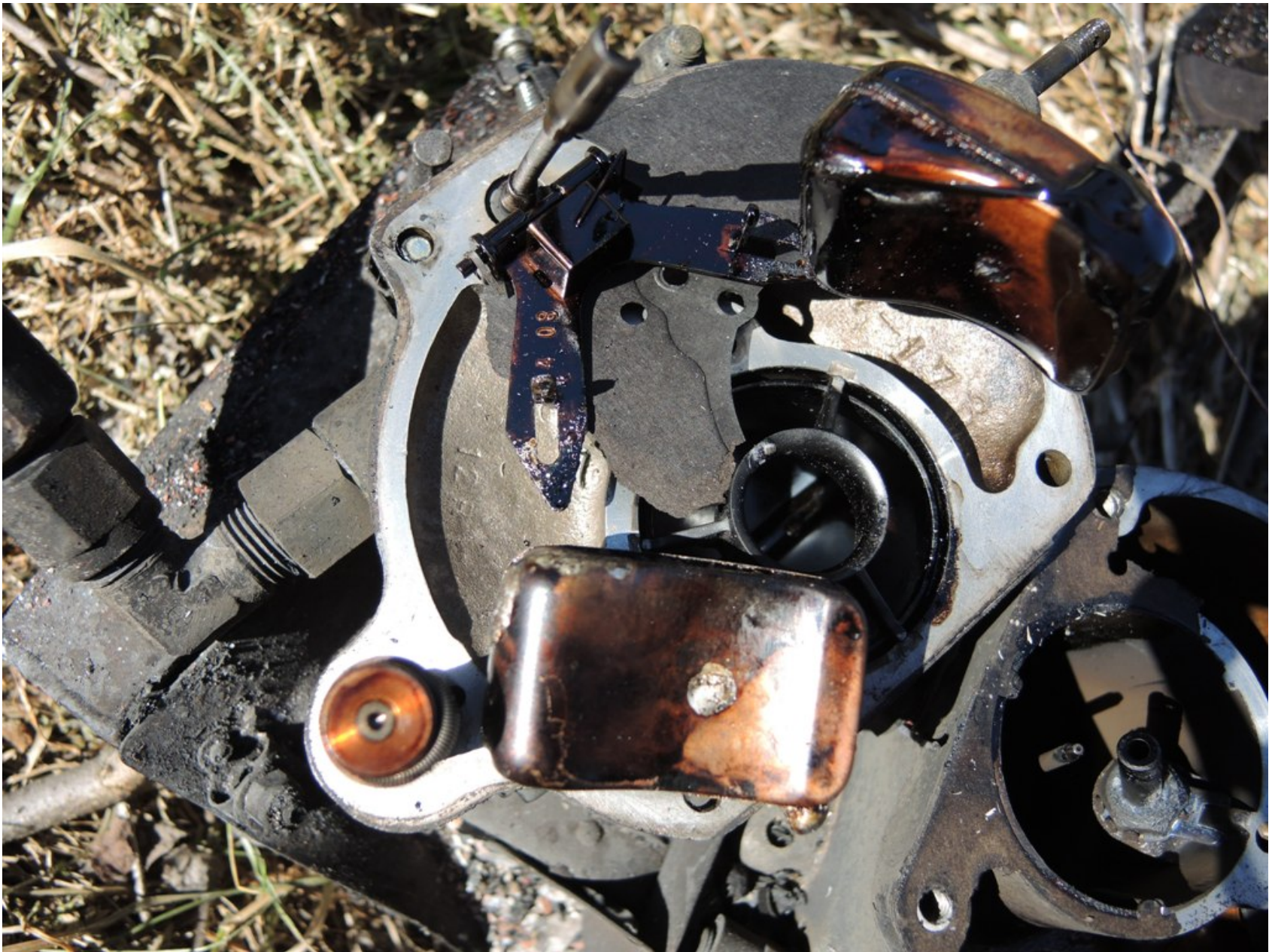
Photo 12 - Textron Aviation Digital Photograph. View Depicting the Carburetor Float. Note the Separated Float on the Left and the Resolidified Solder On the Bottom of the Separated Float.
