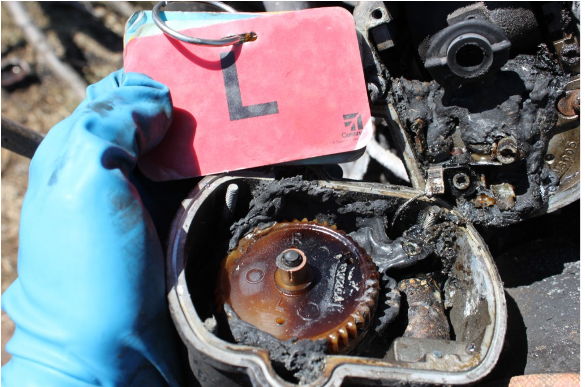
Photo 14 - NTSB Digital Photograph. View of the Internals Of the Left Magneto.
