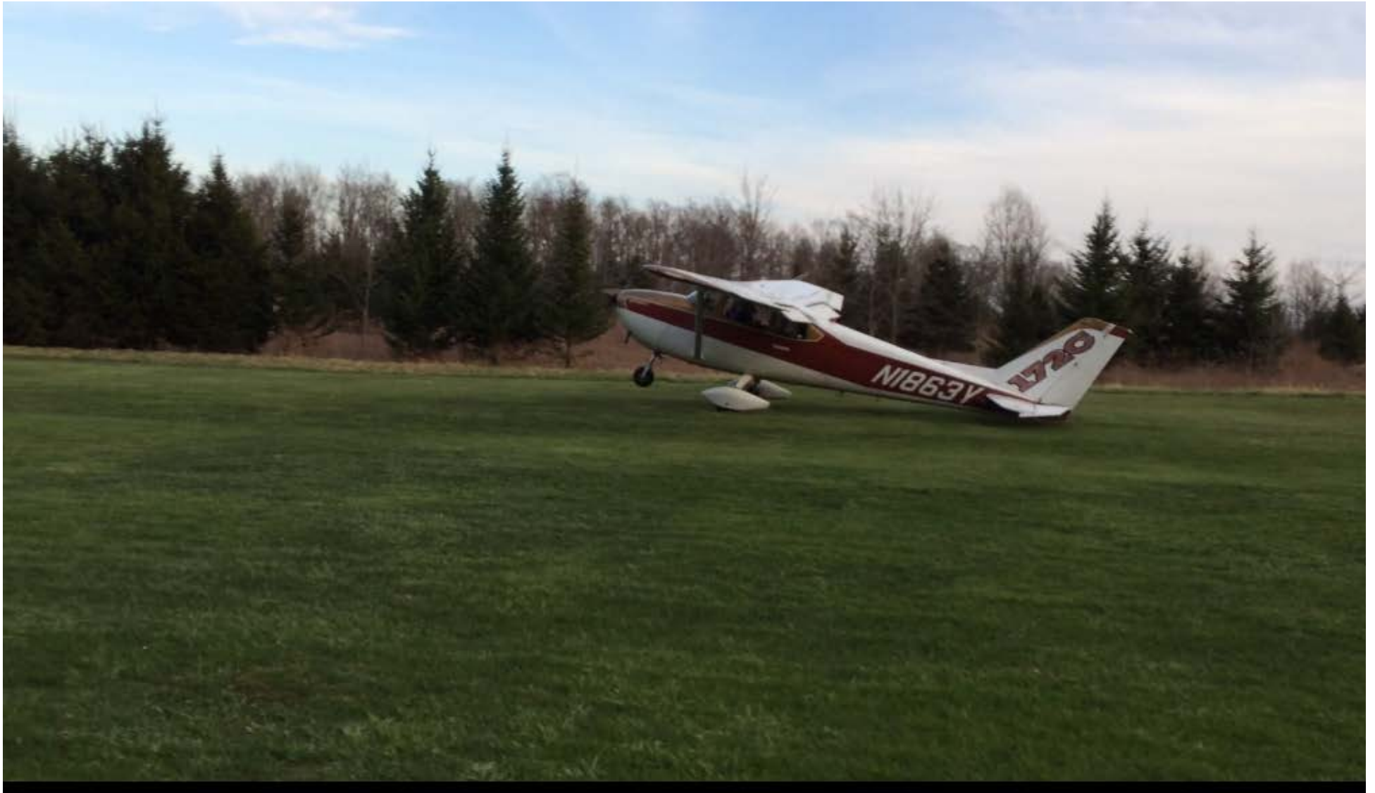
Photo 3 - Screenshot from Video Taken by Airstrip Owner. Left Side View Taken Abeam Camera Operator Location. Note the Position of the Flaps and Elevator
