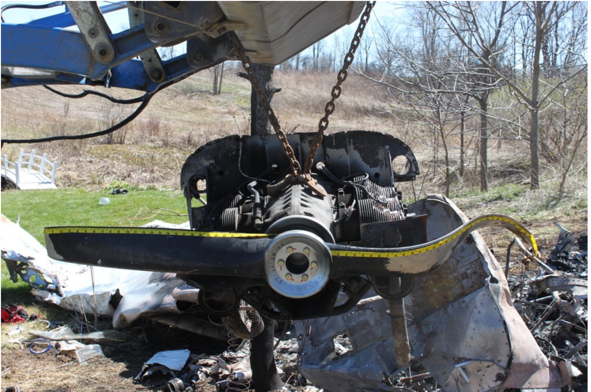
Photo 11 - NTSB Digital Photograph. View of the Propeller and Engine Assembly. Note the Fractured Blade on the Left and Deformed Blade on the Right.
