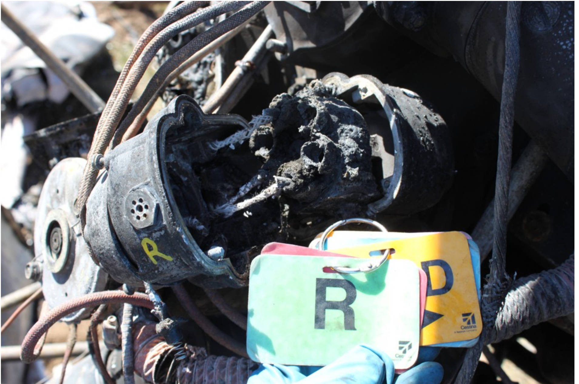
Photo 15 - NTSB Digital Photograph. View of the Internals Of the Right Magneto.
