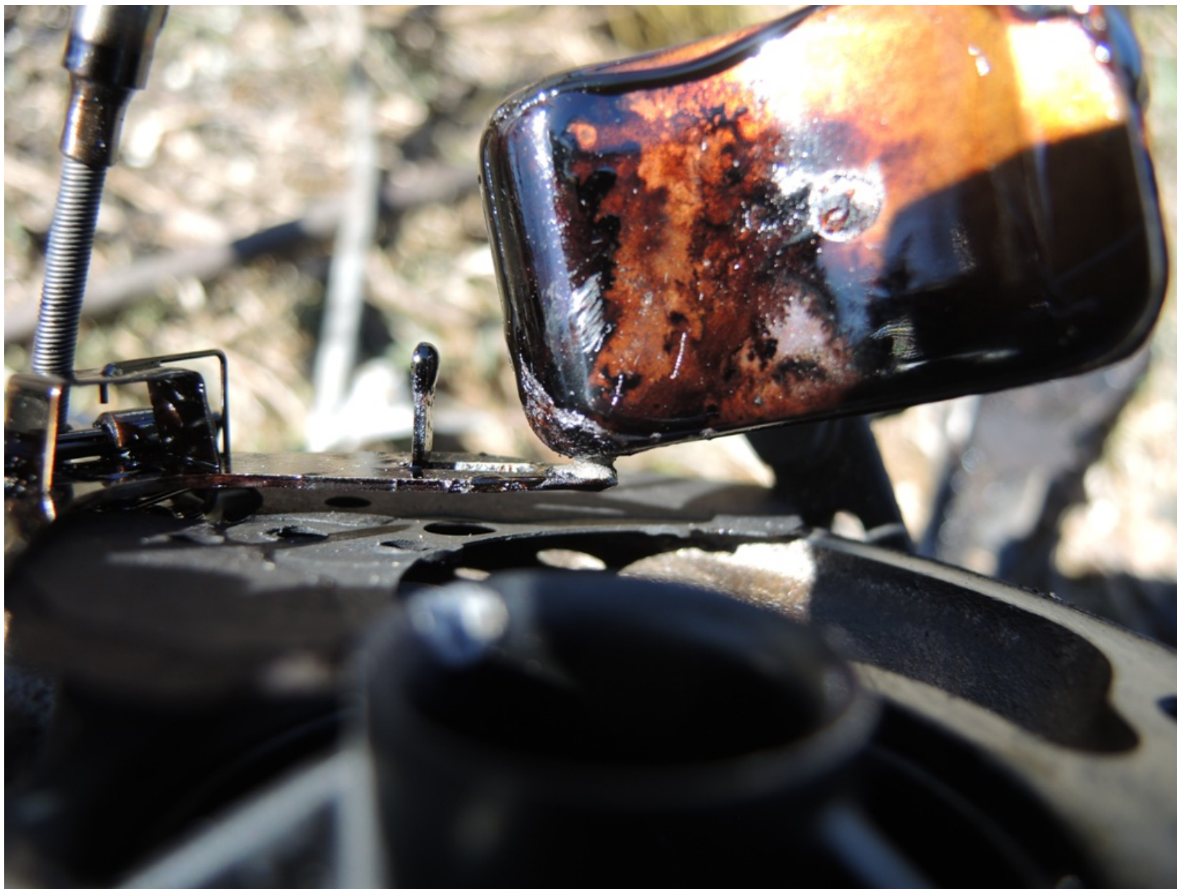
Photo 13 - Textron Aviation Digital Photograph. View Depicting the Attached Carburetor Float and the Solder Joint. Note the Discoloration of the Float.
