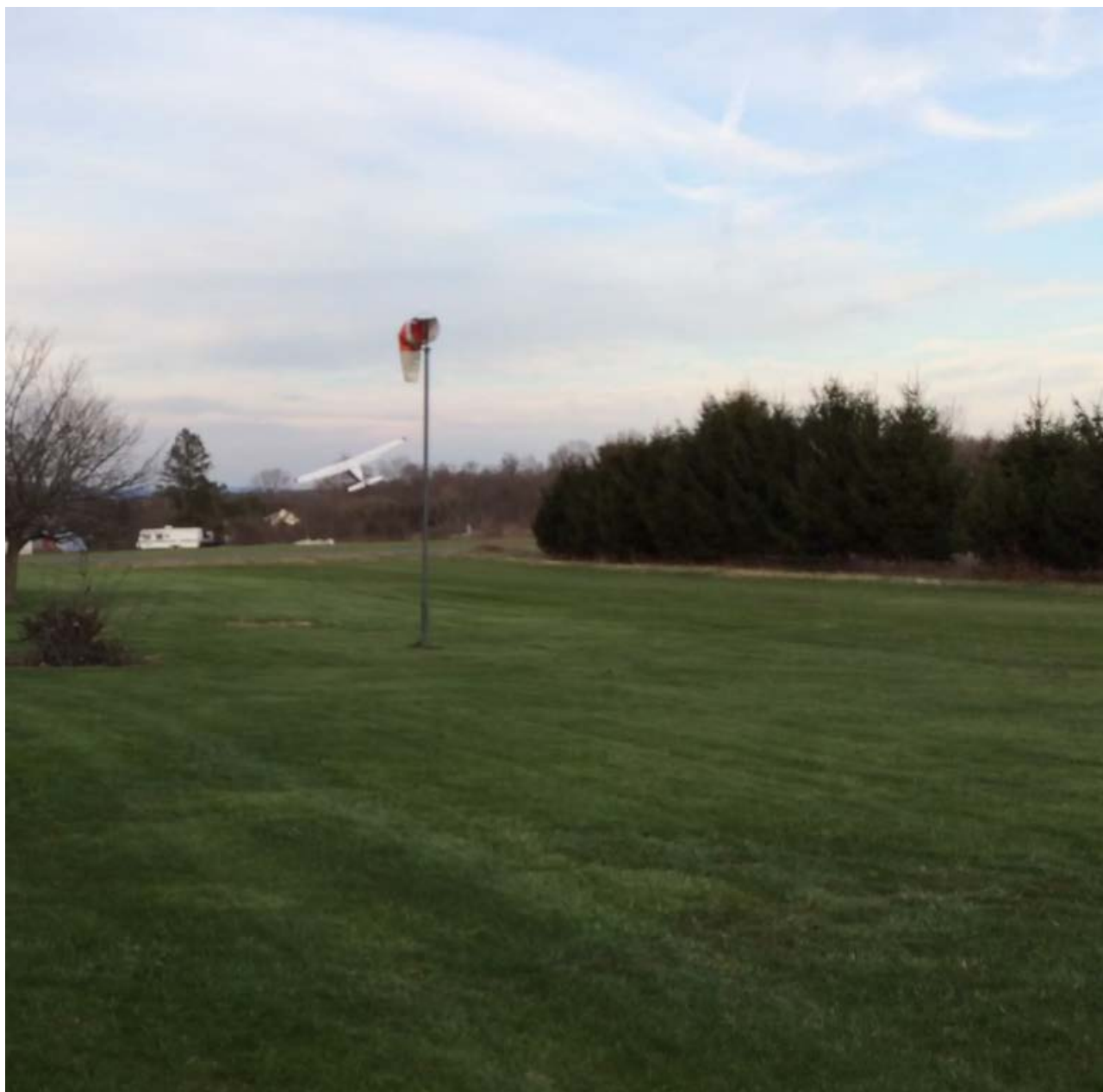
Photo 5 - Screenshot from Video Taken by Airstrip Owner. Rear View Depicting the Airplane in a Left Roll and Nose-High Attitude While Airborne Past the Windsock. Note the Windsock Depicting The Wind From the West.
